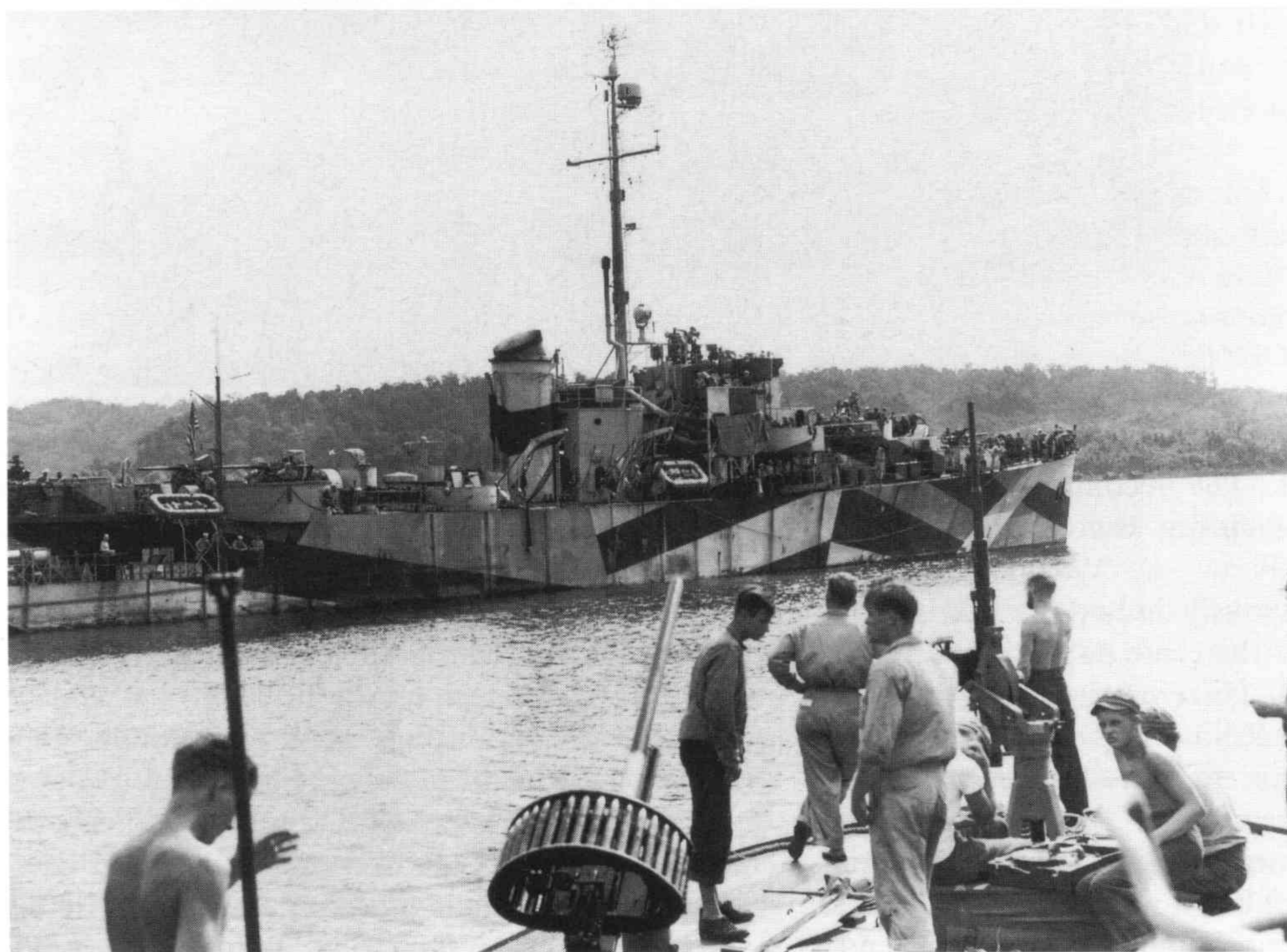
20mm Oerlikon (furthest from camera) and 37mm M4 on US PT Boat in 1944. Note the continuous-belt feed forming a hoop over the M4 (Courtesy: US Naval Historical Centre)
