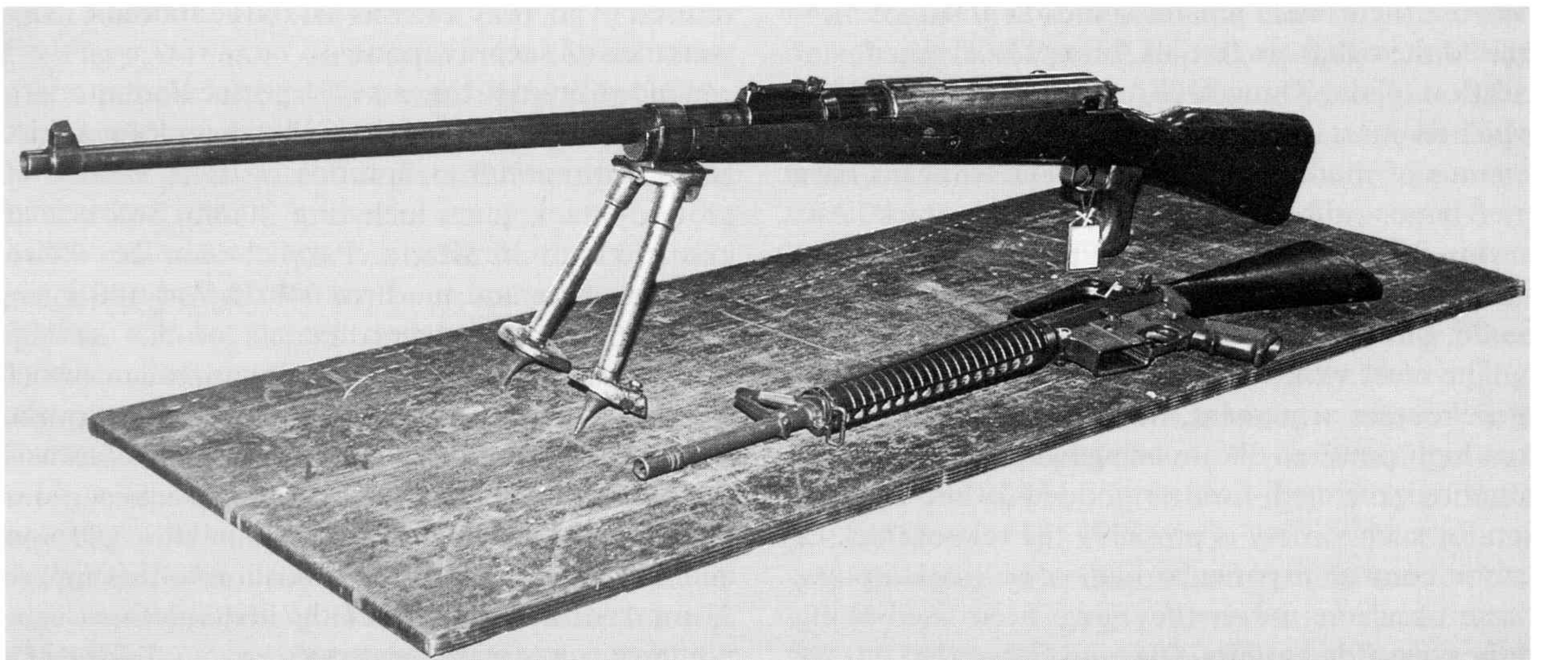
Mauser Tank-Gewehr M1918 (with M16 rifle for comparison) (Courtesy: MoD Pattern Room)
