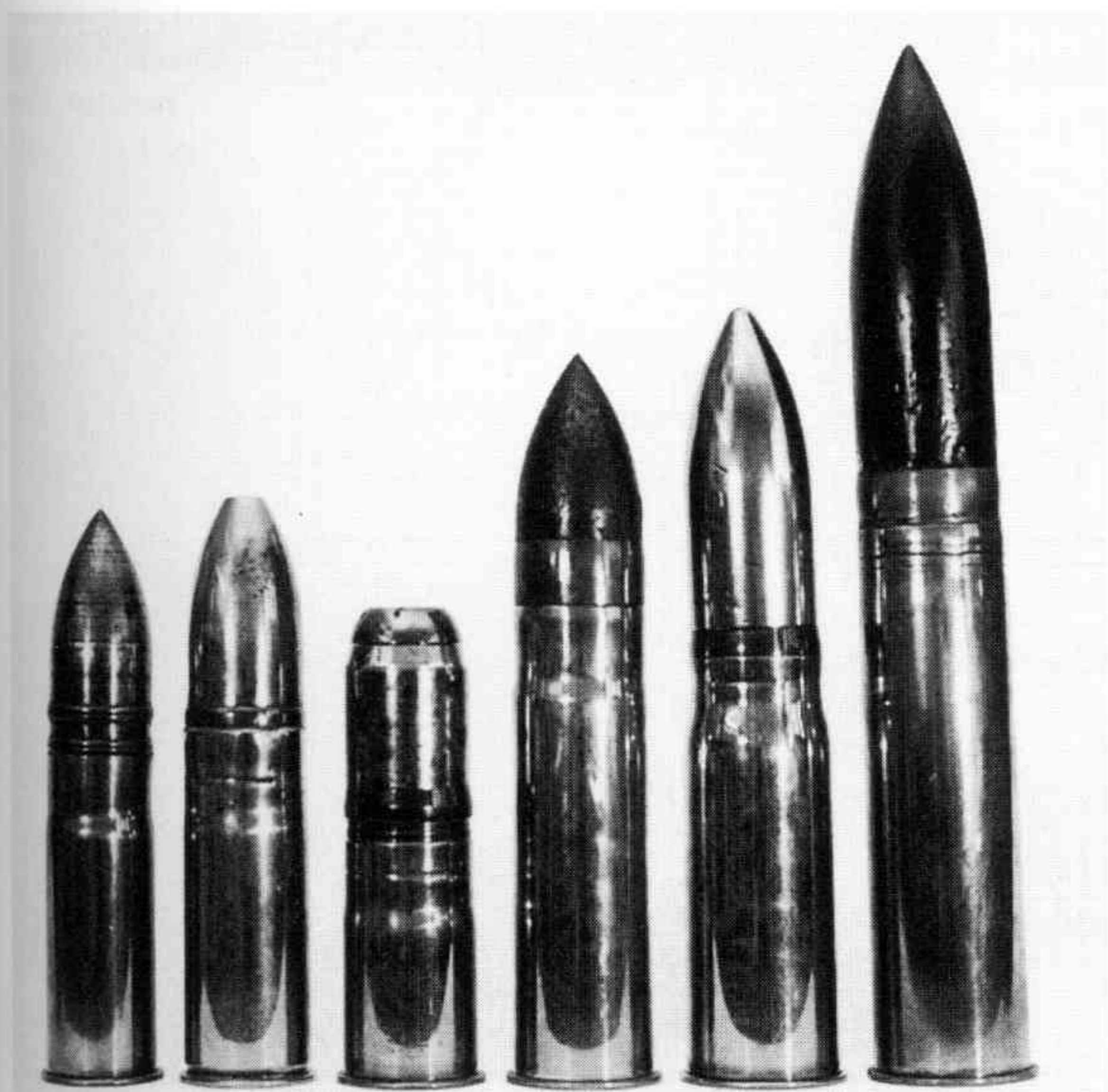
The 'Pom-pom' family of cartridges (from left to right): 37mm Maxim (37 × 94R), 3.7cm Sockelflak (37 × 101SR), 1pdr Vickers Mk III (37 × 69R), USN Heavy One-Pounder (37 × 137R), 1½pdr Vickers (37 × 123R), 2pdr Vickers (40 × 158R)
