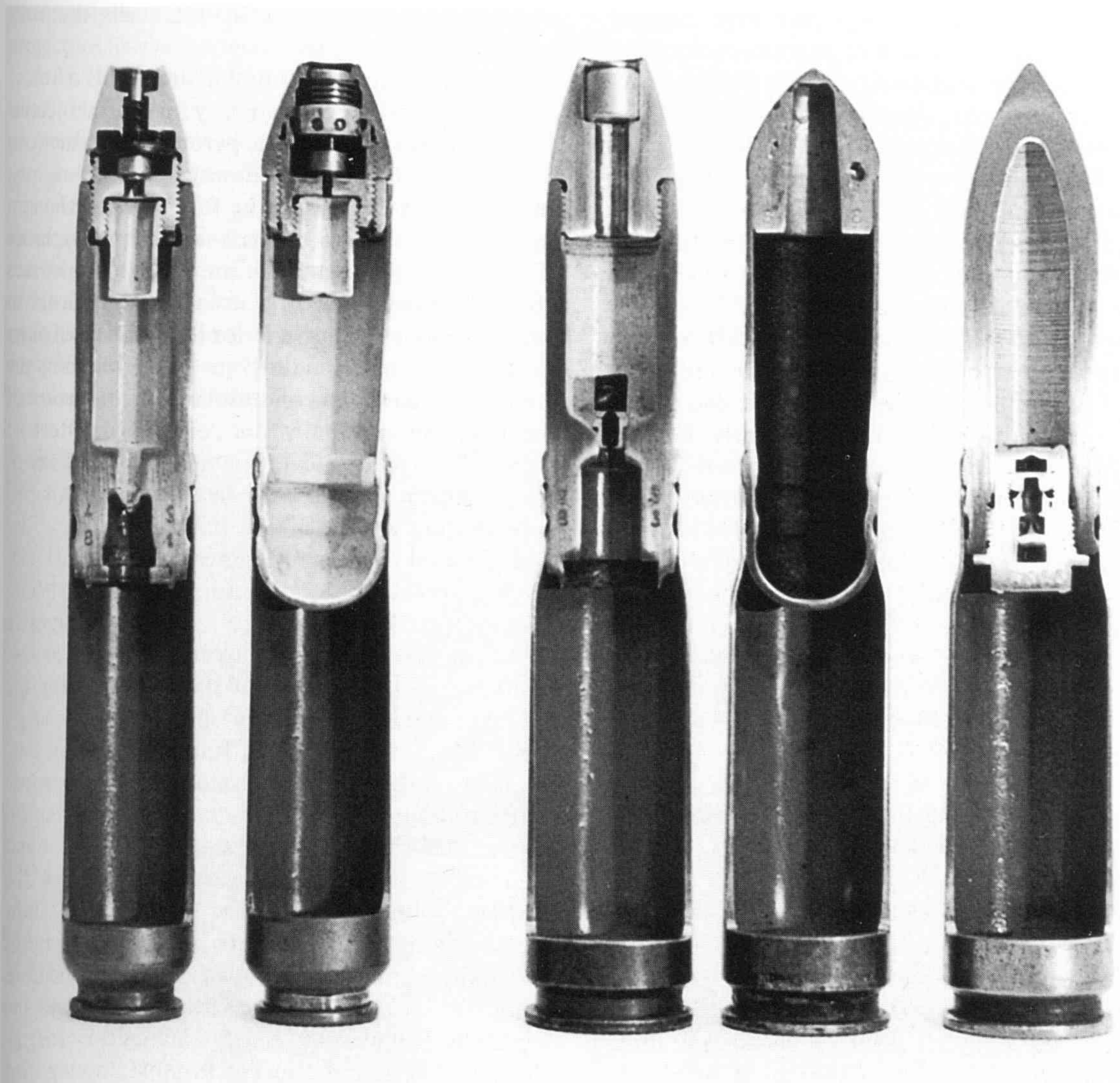
Sectioned German WW2 aircraft gun cartridges (from left to right): 20 × 80RB HE/T-SD for MG-FF, 20 × 80RB HE (M-Geschoss) for MG-FFM, 20 × 82 HE/T-SD for MG 151/20, 20 × 82 HE (M-Geschoss) for MG 151/20, 20 × 82 AP/HE (base fuze) for MG 151/20. Note differences between mechanical (1 and 2) and chemical (3) fuzes. Cartridge 4 is a practice round with a dummy fuze.
