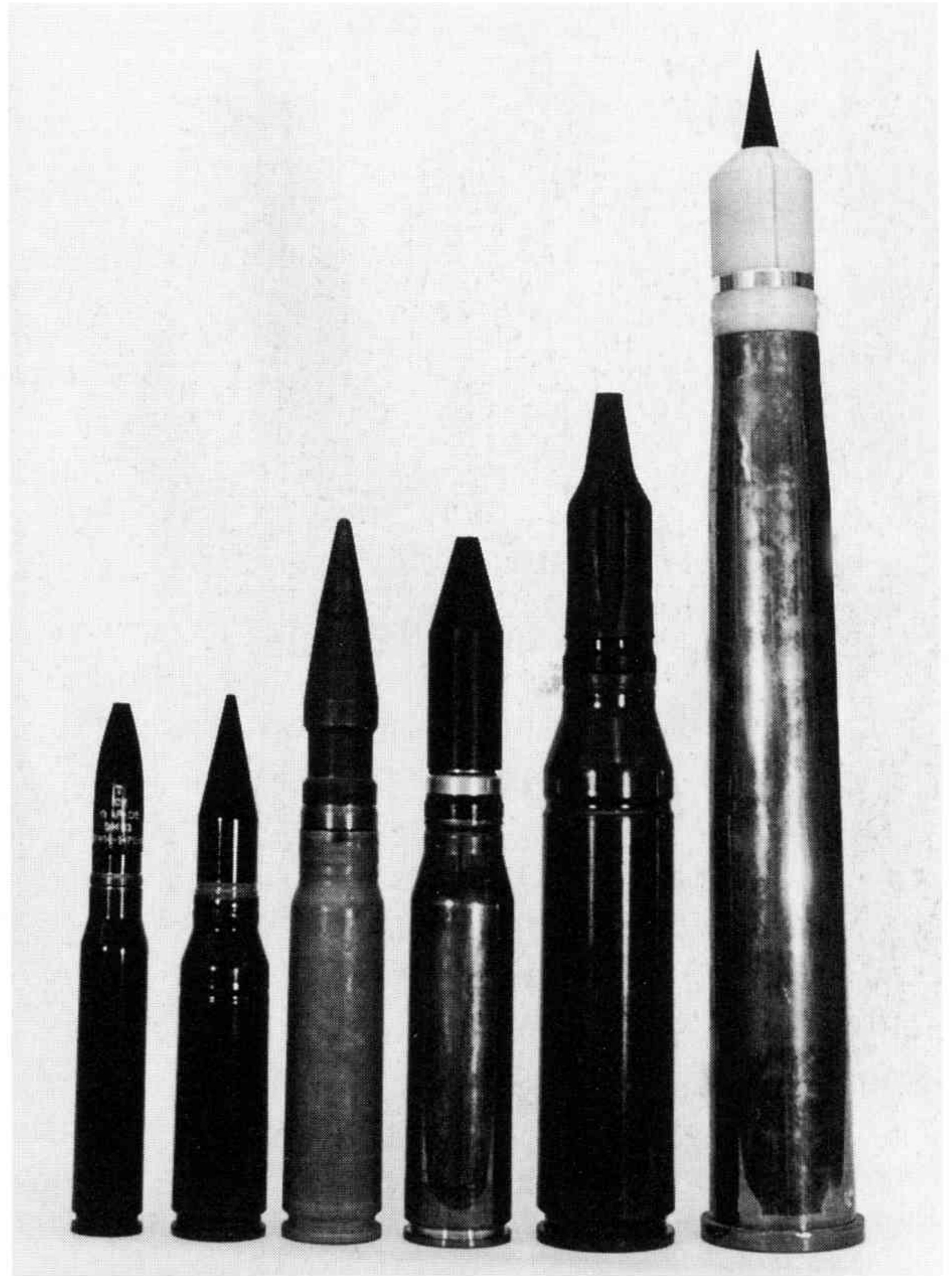
Postwar AFV cartridges (left to right): 20 × 139 APDS (HS820, Oerlikon KAD, Rh202); 25 × 137 AP (Oerlikon KBA); 30 × 165 APHE (2A38/42/72); 30 × 170 APDS (Rarden); 35 × 228 APDS (Oerlikon KD series); 40 × 364R with experimental APDS (Bofors)
