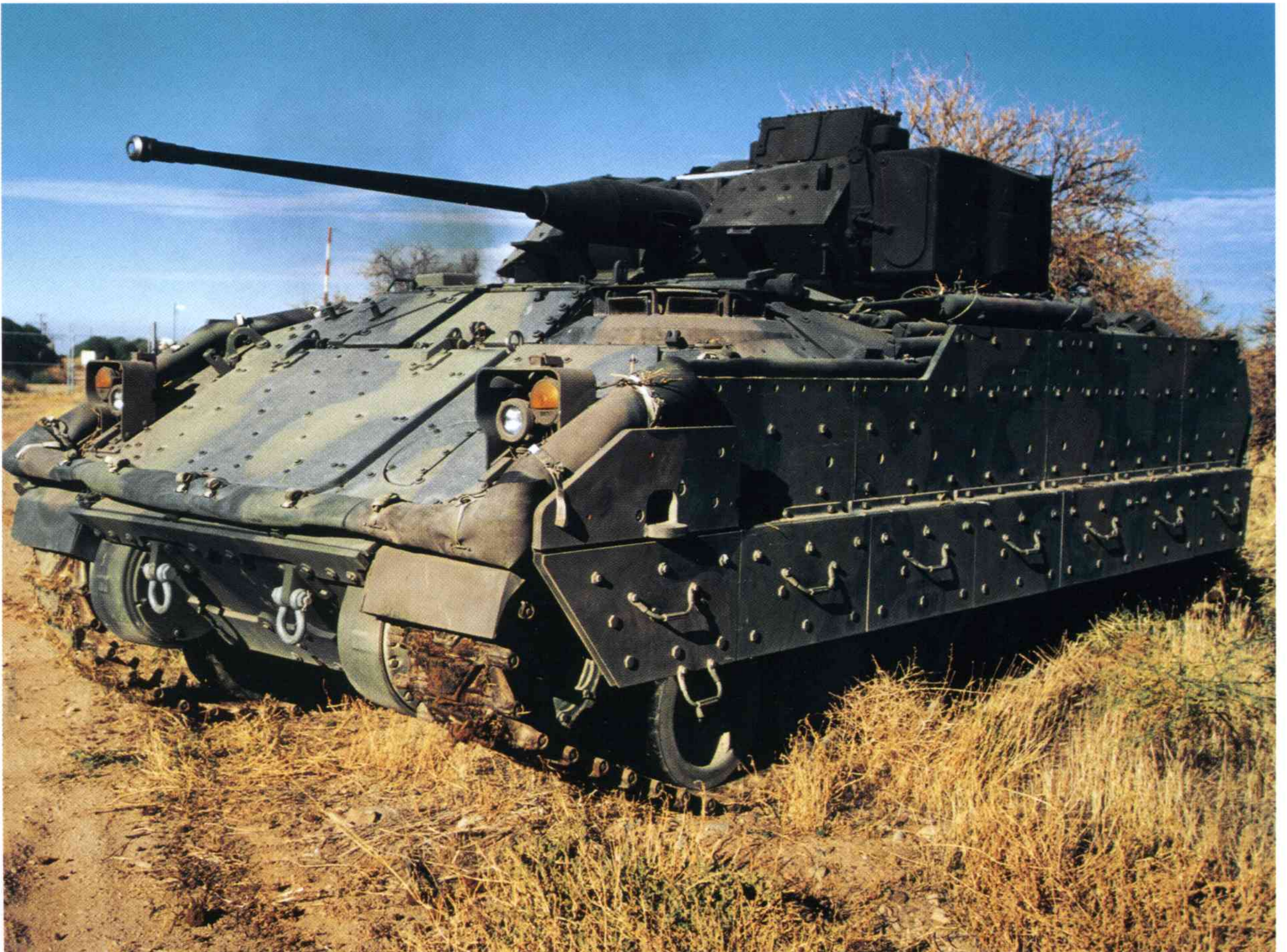
35/50mm Bushmaster III Chain Gun on M2 Bradley MICV (Courtesy: MDHC)
