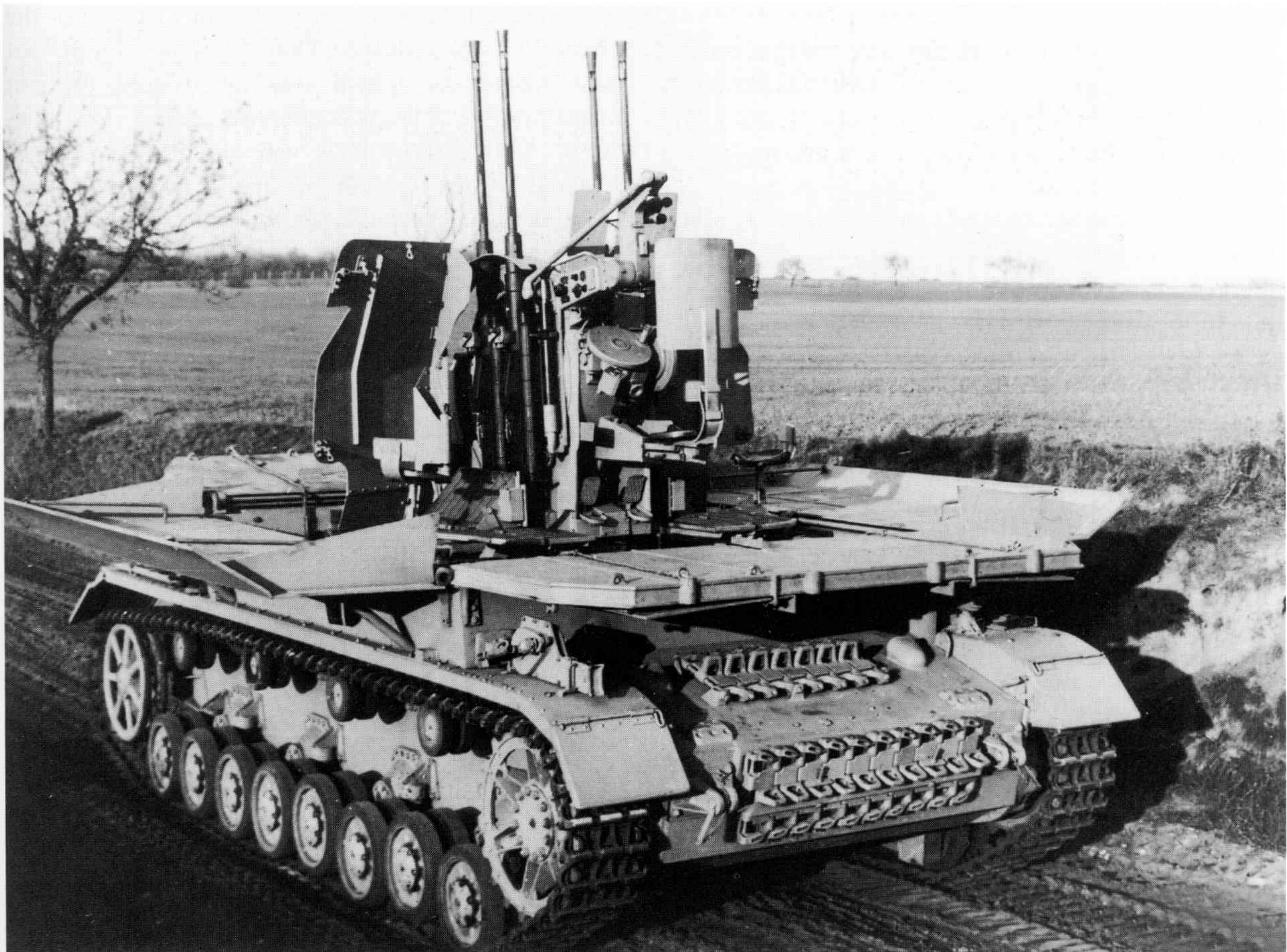
Flakpanzer IV (2cm): 2cm Vierlingsflak 38 on chassis of Pz IV (Imperial War Museum)
