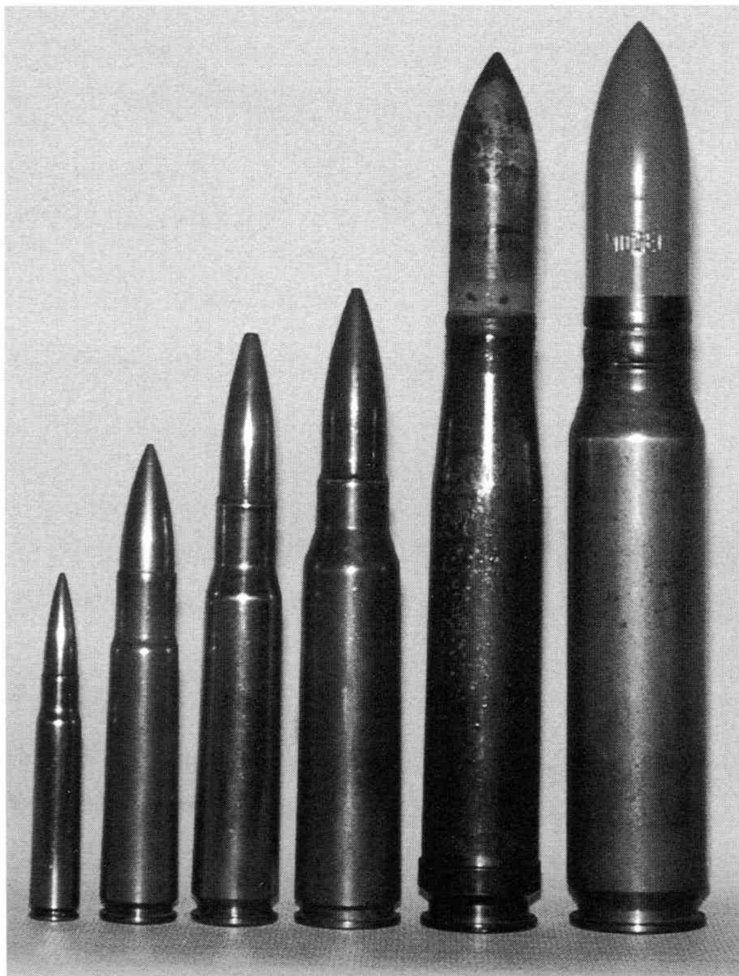
World War 2 AFV gun cartridges (left to right): 7.92 × 57 (for scale), .5" Vickers (12.7 × 81), .50" Browning (12.7 × 99), 15mm Besa (15 × 104), KwK 30/38 (20 × 138B), Swiss Pzw. Kan. 38 (24 × 138)
