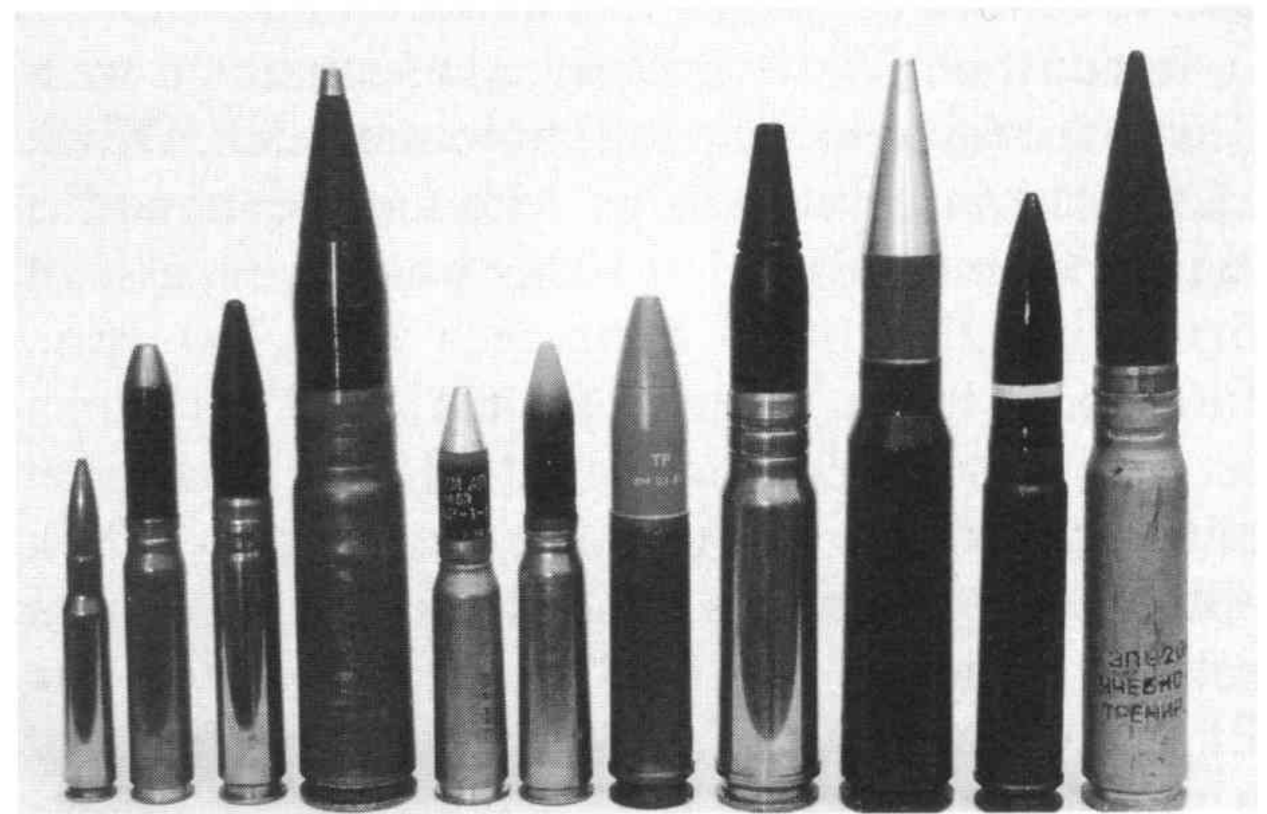
Postwar fighter gun cartridges (from left to right): .50" M3 ( 12.7 \times 99 ), 20mm Hispano/M3/M24 ( 20 \times 110 ), Soviet NS-23/NR-23/GSh-23 ( 23 \times 115 ), Soviet N-37 ( 37 \times 155 ), US M39/M61 ( 20 \times 102 ), USN Mk 11/Mk 12 ( 20 \times 110 ), 30mm Aden/DEFA + M230 chain gun ( 30 \times 113B ), Soviet NR-30 ( 30 \times 155B ), Oerlikon KCA ( 30 \times 173 ), Mauser BK 27 ( 27 \times 145B ), Soviet GSh-30/GSh-6-30/GSh-301 + 2A42 helicopter gun ( 30 \times 165 )
