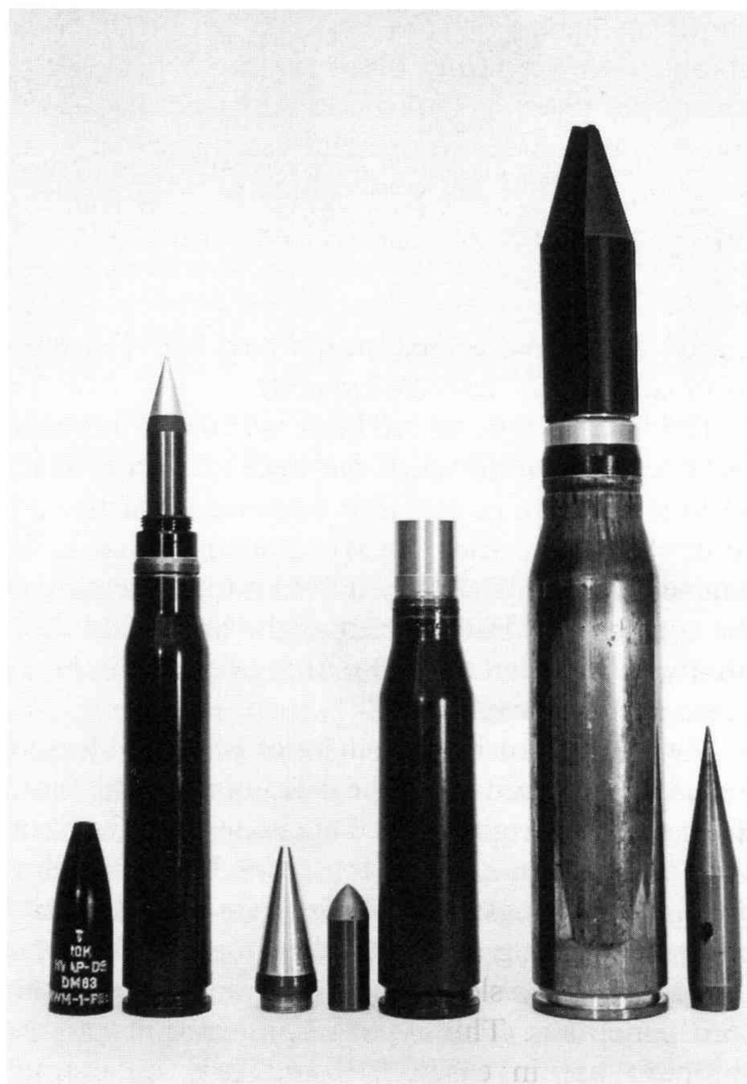
Armour-piercing technology (from left to right): APDS for 20 × 139 with plastic sabot removed, APCR for 20 × 128 with alloy nose-cone and tungsten core removed, APDS for 30 × 170 (Rarden) with sharply-pointed tungsten core
