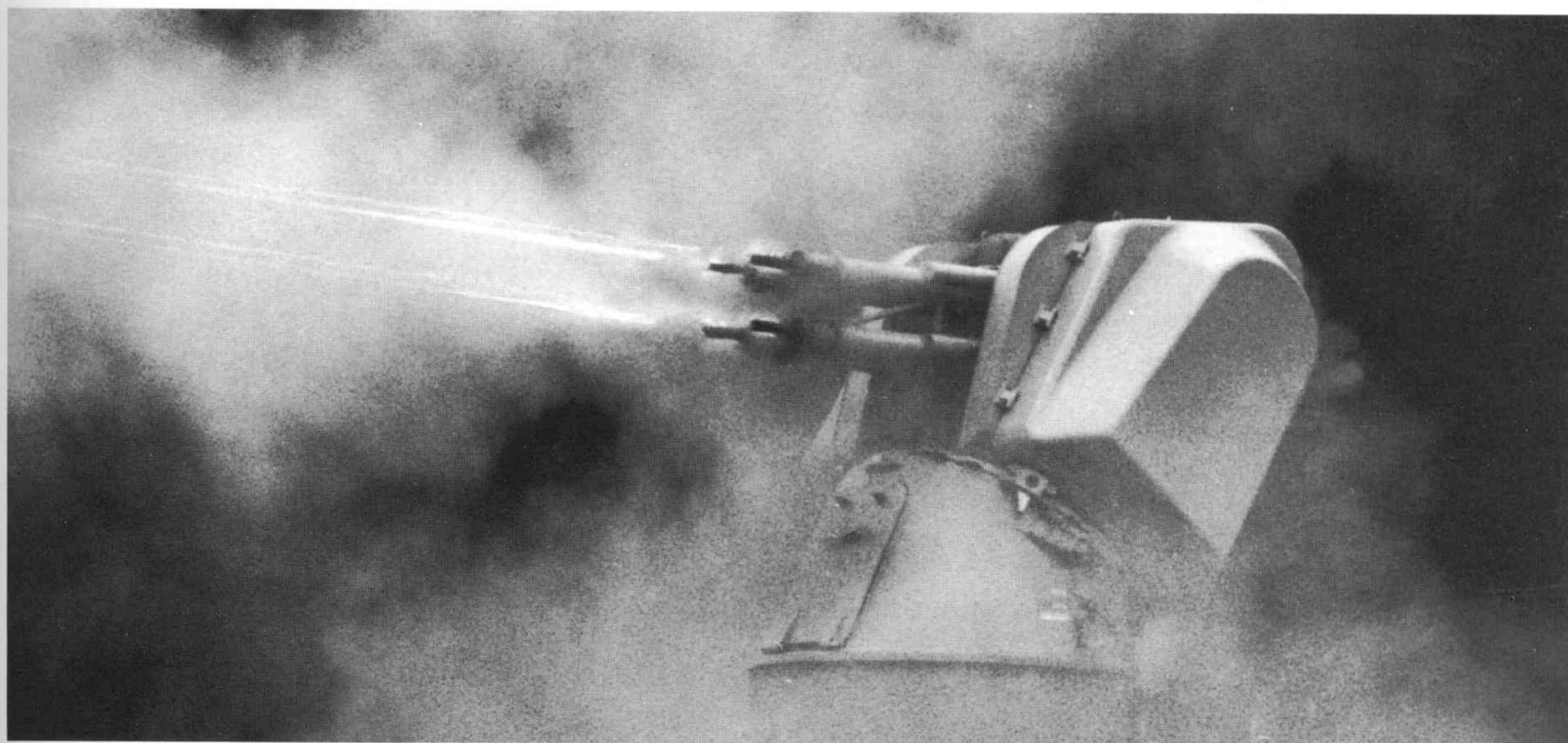
Oerlikon Sea Zenith CIWS with four 25mm KBB cannon (Courtesy: Oerlikon/Ian Hogg)
