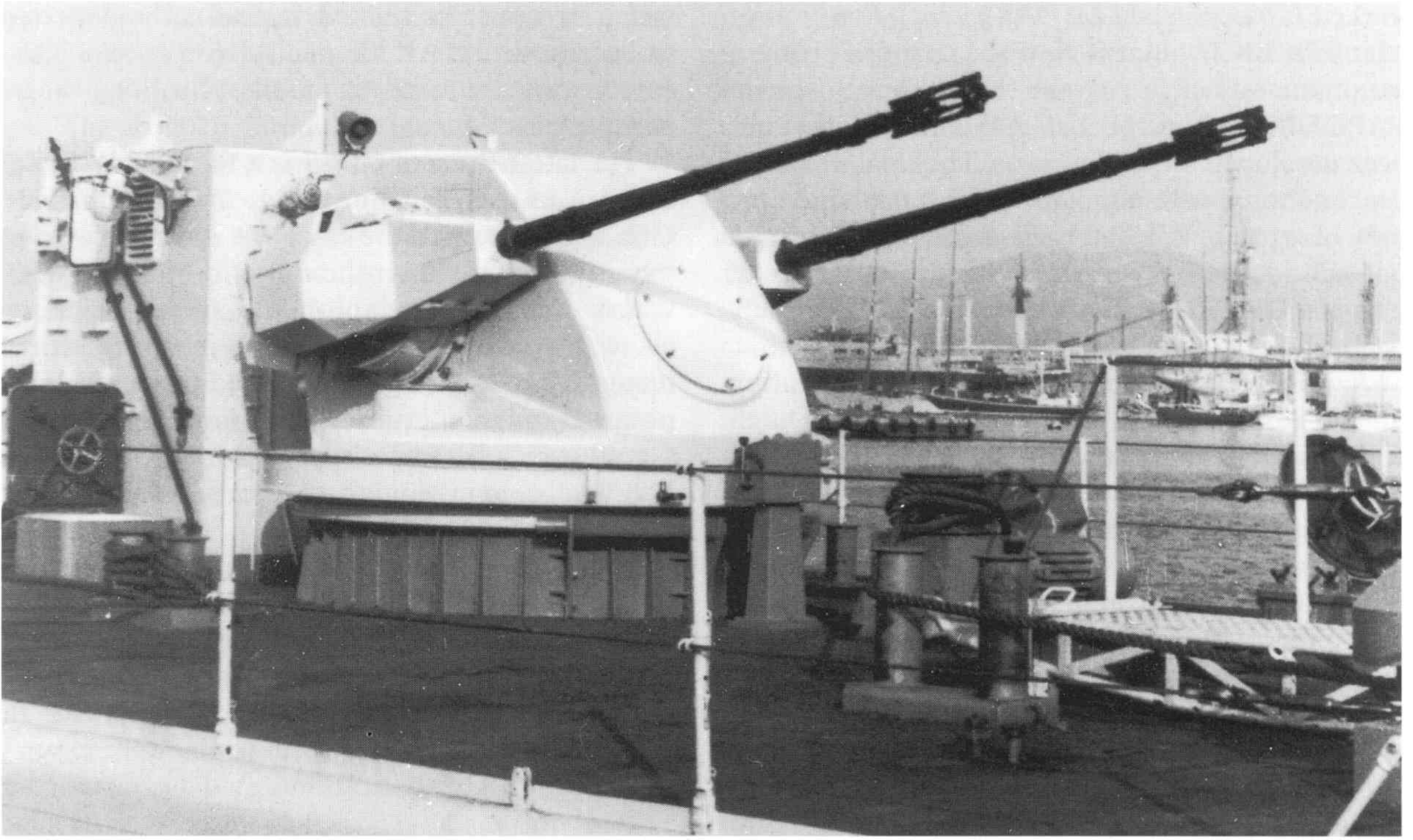
OE/OTO mounting with twin 35mm Oerlikon guns (Courtesy: Oerlikon/Ian Hogg)
