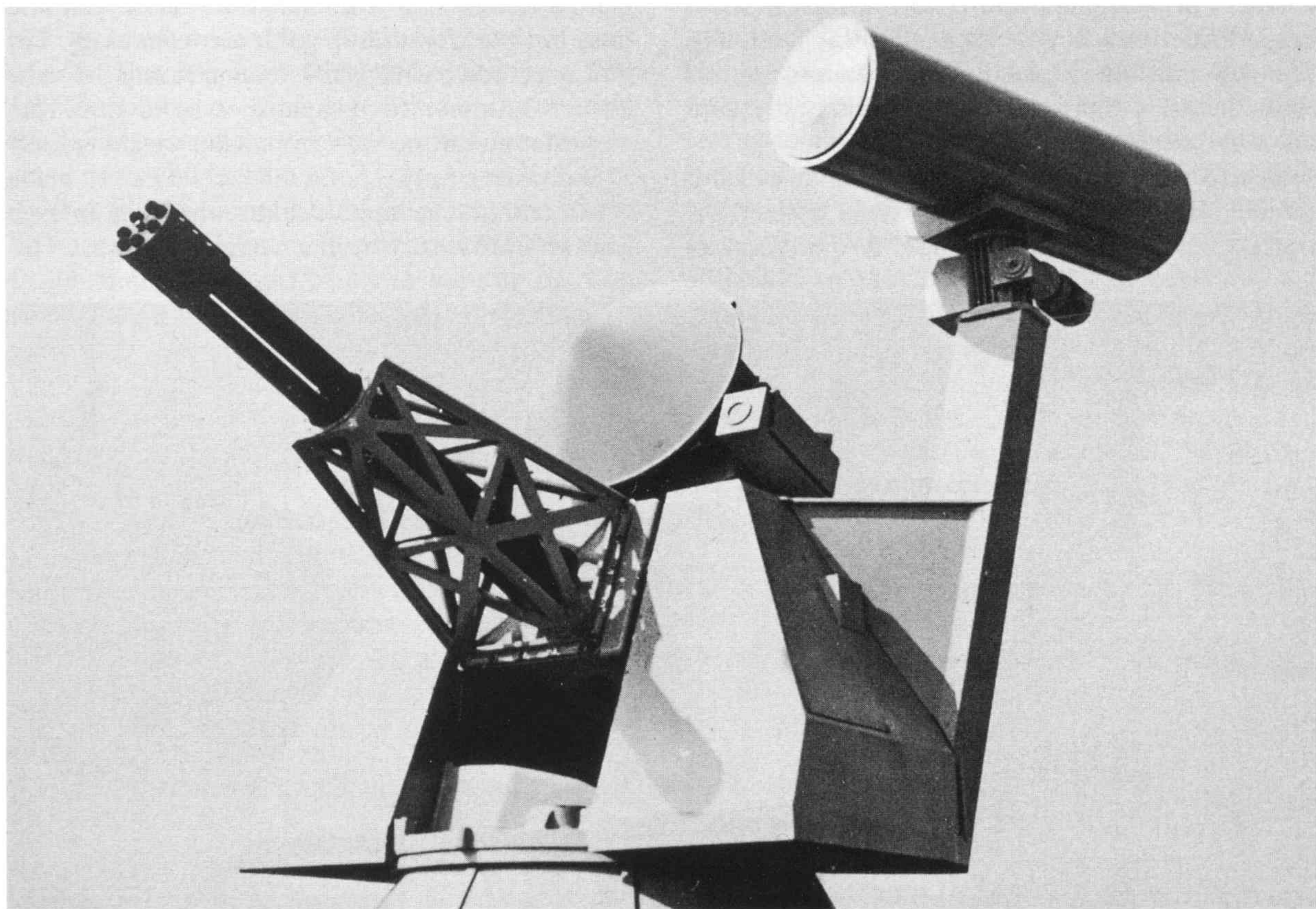
Goalkeeper CIWS with 30mm GAU-8/A (Courtesy: MoD Pattern Room)
