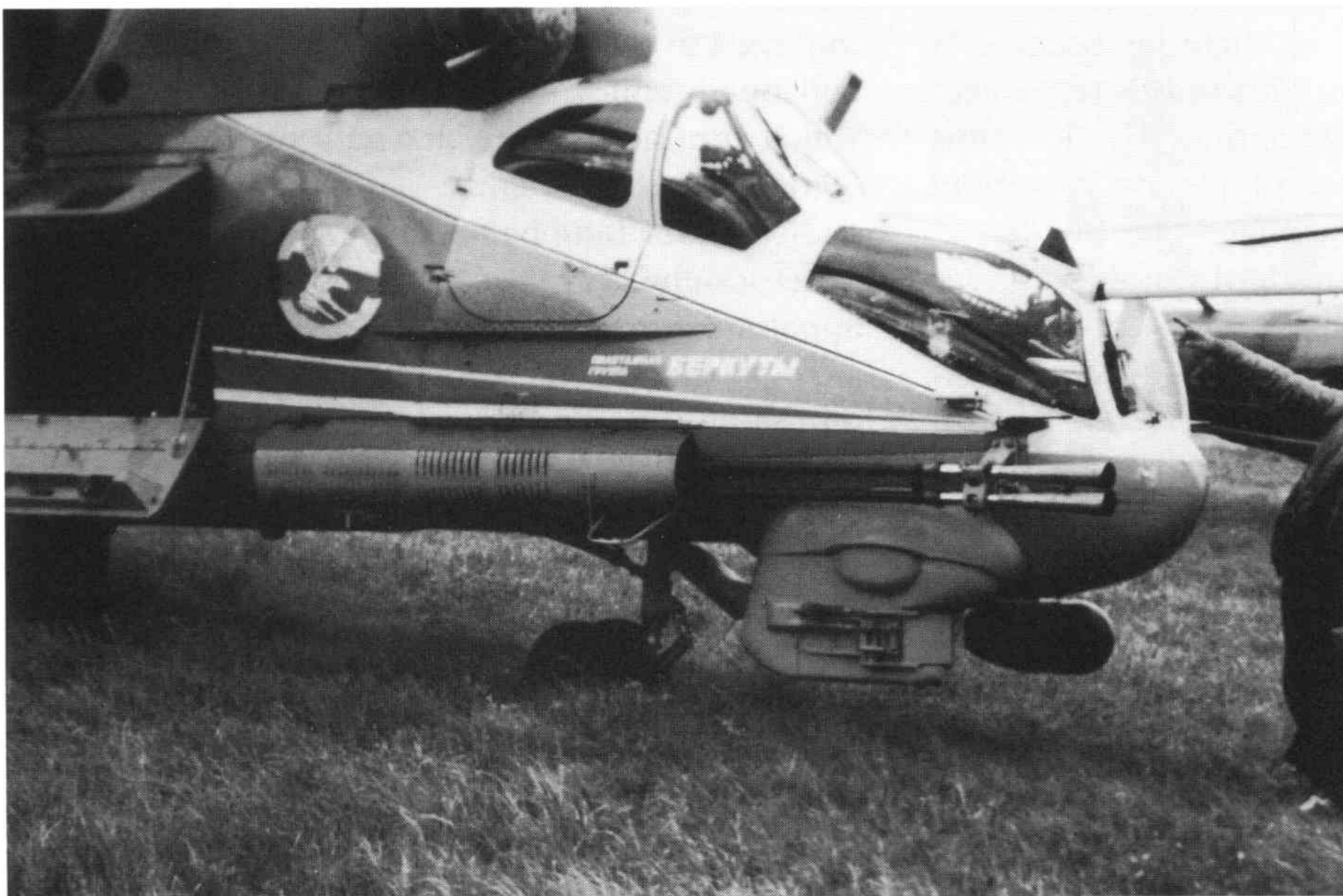
YakB-12.7 four-barrel rotary gun in Mi-24 Hind-D (Courtesy: MoD Pattern Room)
