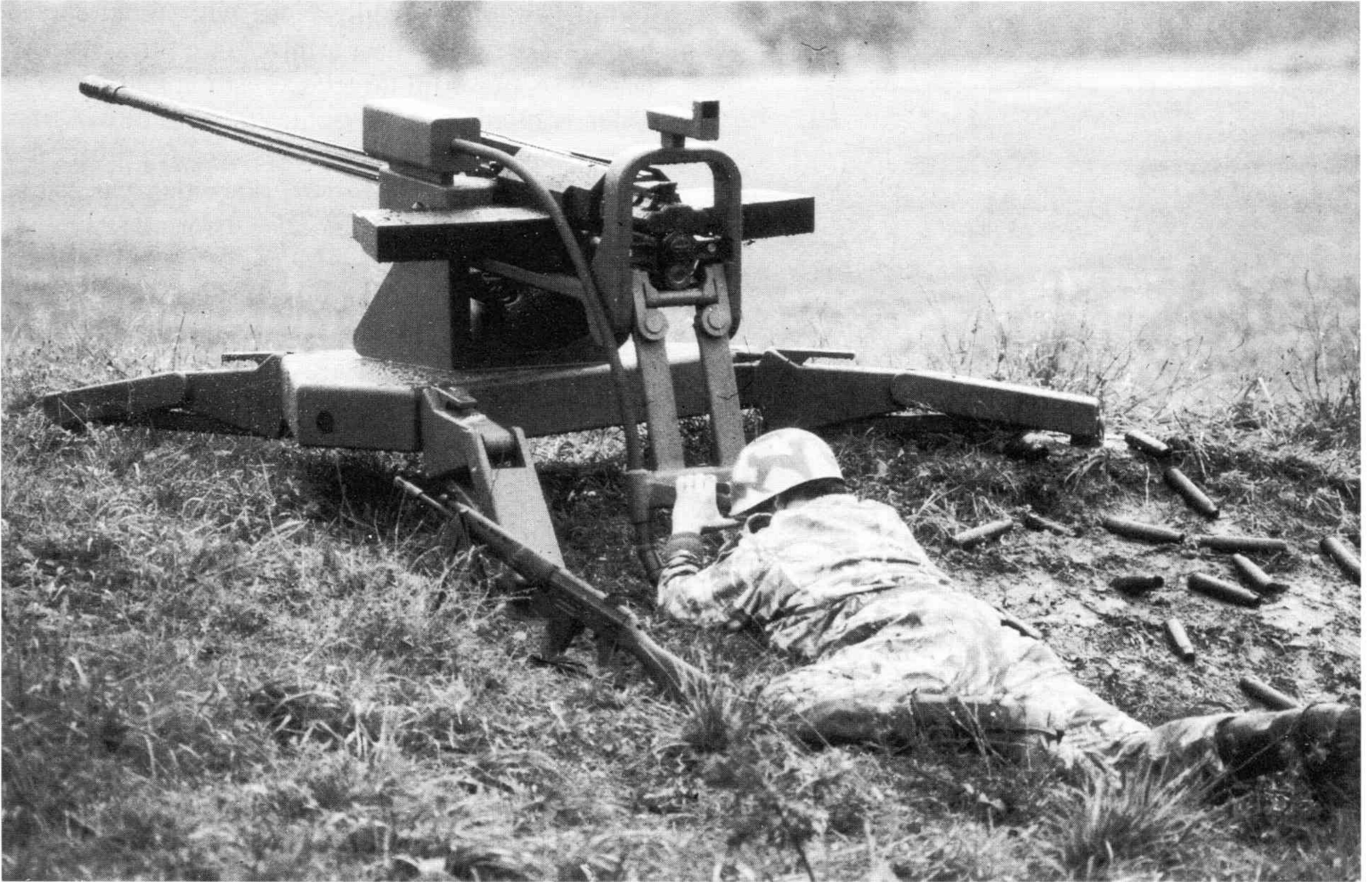
Oerlikon ILTIS mounting (25mm KBB gun) (Courtesy: Oerlikon-Contraves/Ian Hogg)
