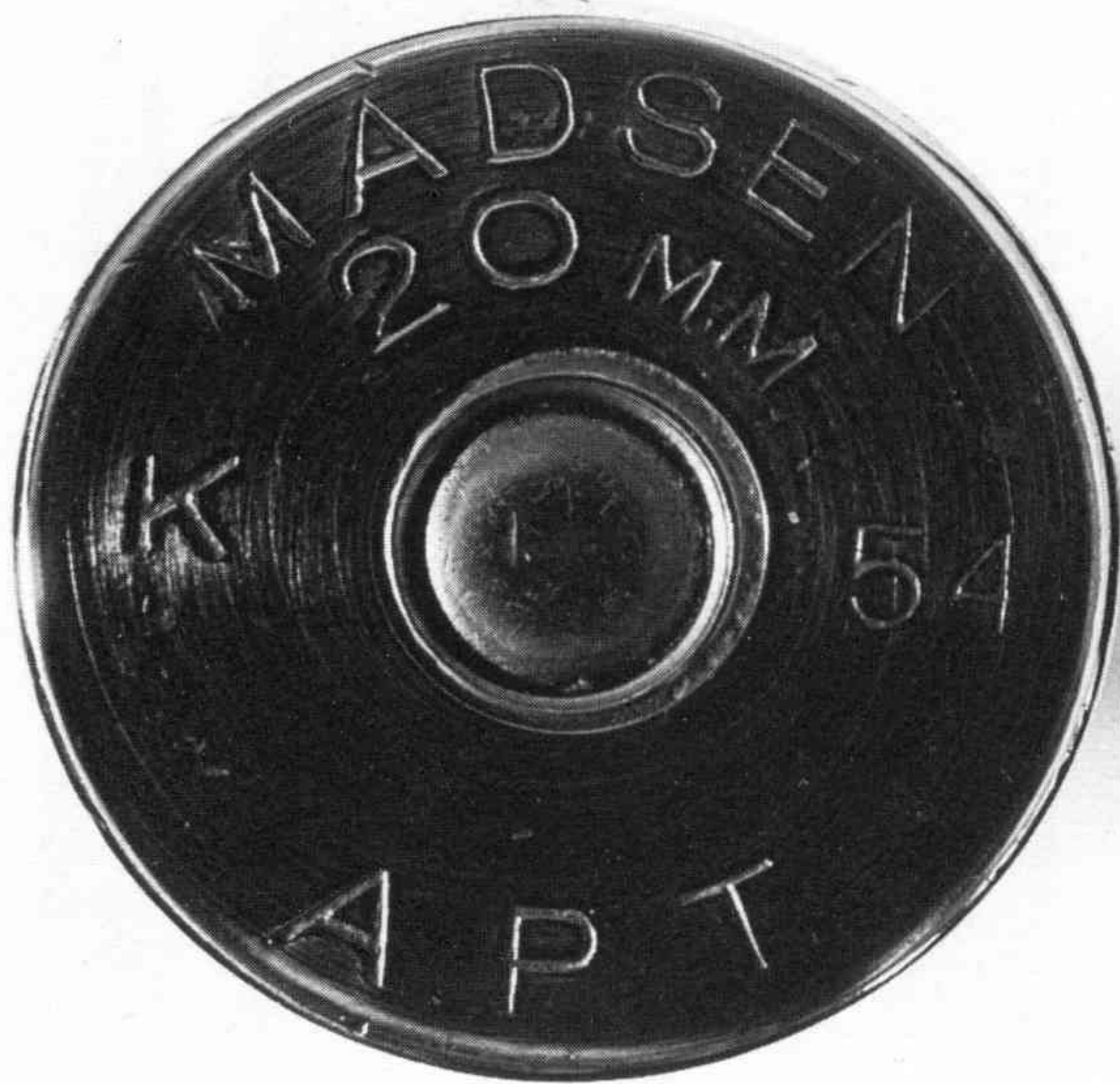
Headstamp for 20mm Madsen, made by Kynoch in 1954 and loaded with an armour-piercing tracer projectile (not all headstamps are so helpful!)
