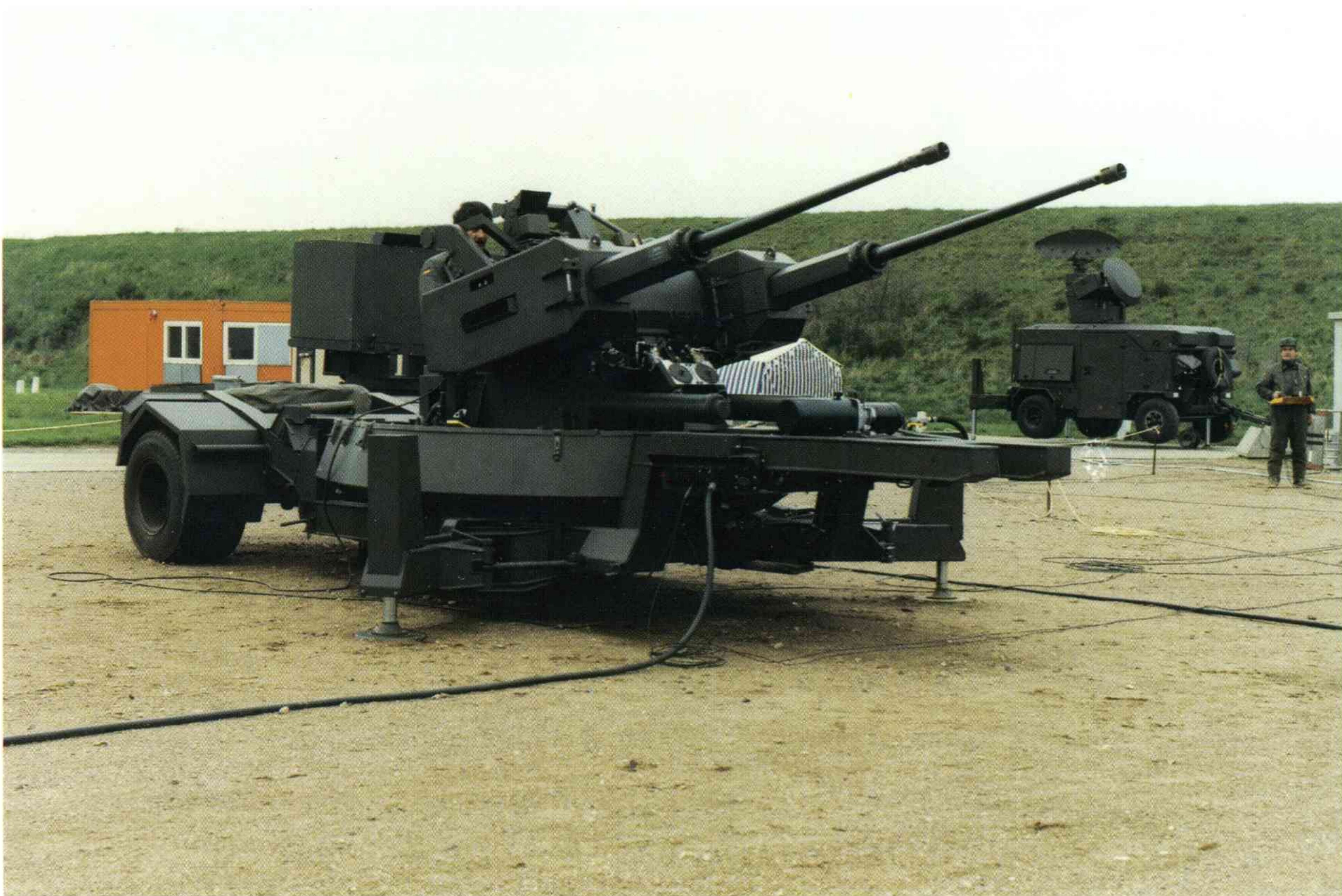
Arrow AA system (two 30mm Mauser MK30F) (Courtesy: Mauser)
