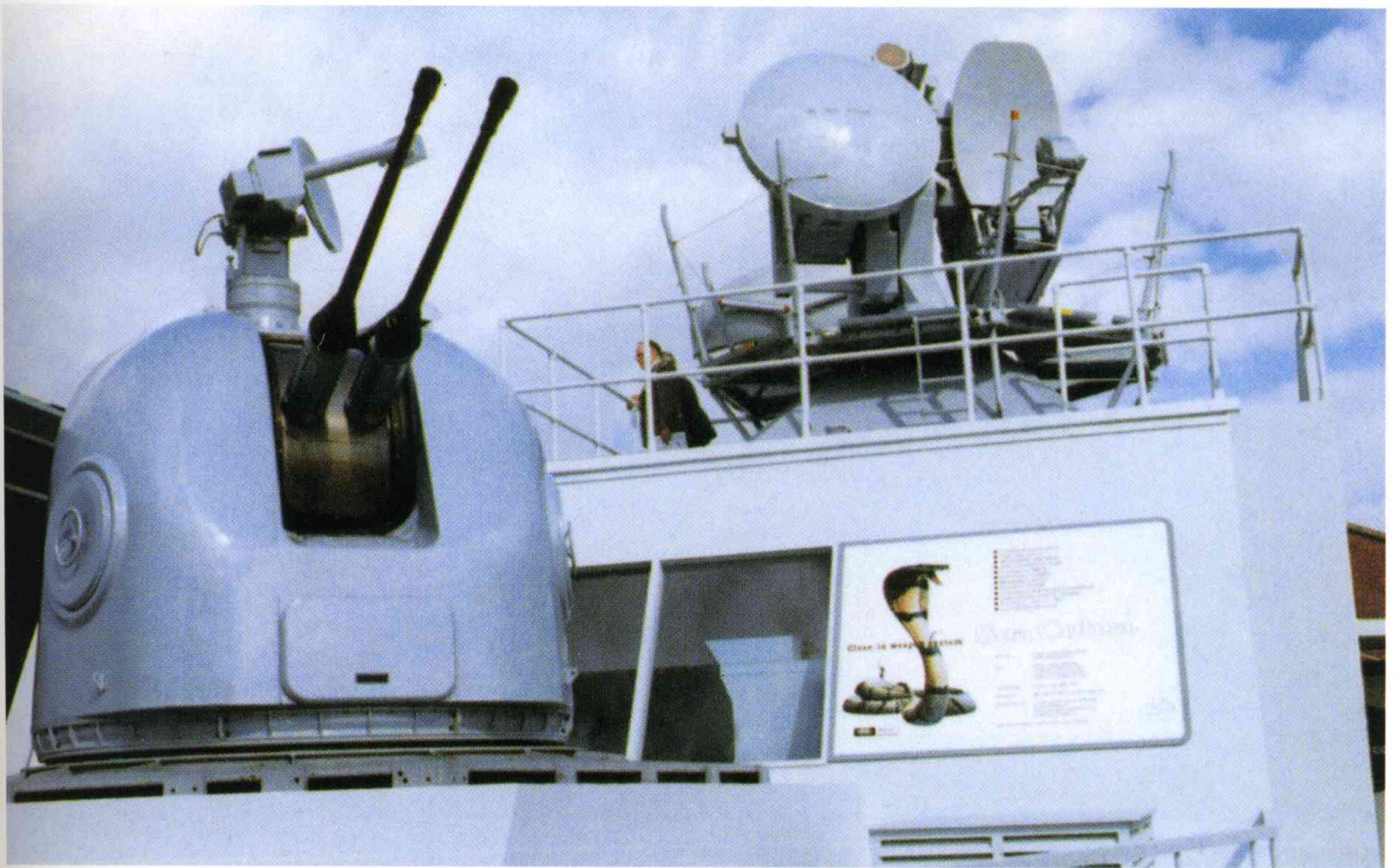
Sea Cobra CIWS with twin Mauser MK30 (Leo Marriott)
