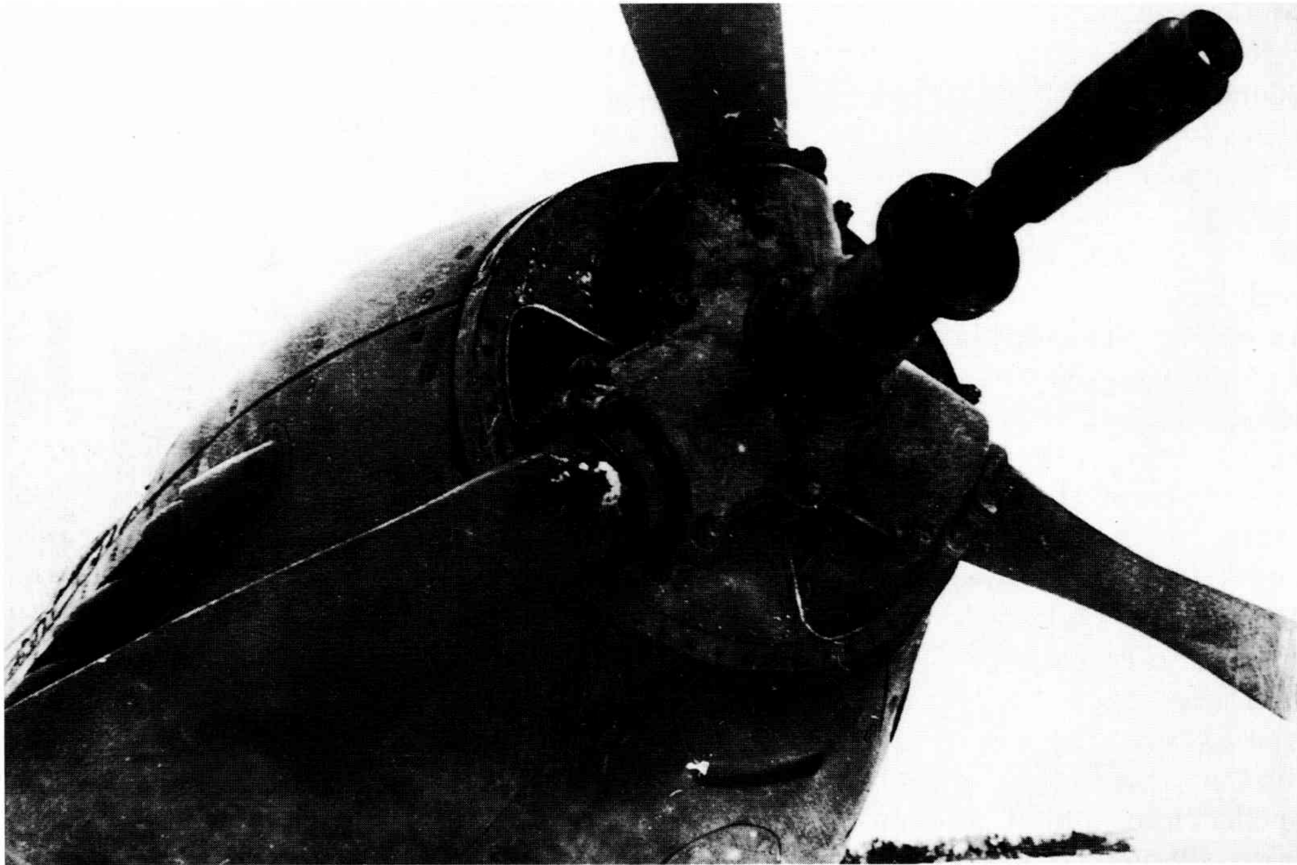
Muzzle brake of an NS-45 protruding from the propeller hub of a Yak-9K (Courtesy: Russian Aviation Research Trust)
