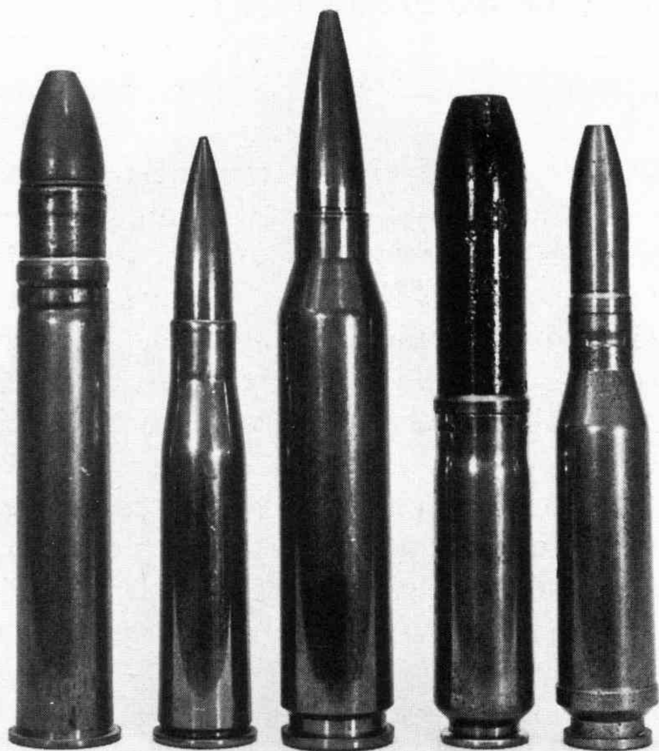
Cartridge case types (from left to right): Rimmed, straight (20 × 99R), Semi-rimmed (13 × 92SR), Rimless, bottle-necked (15 × 115 experimental), Rebated (20 × 72RB), Belted (13 × 93B experimental)
