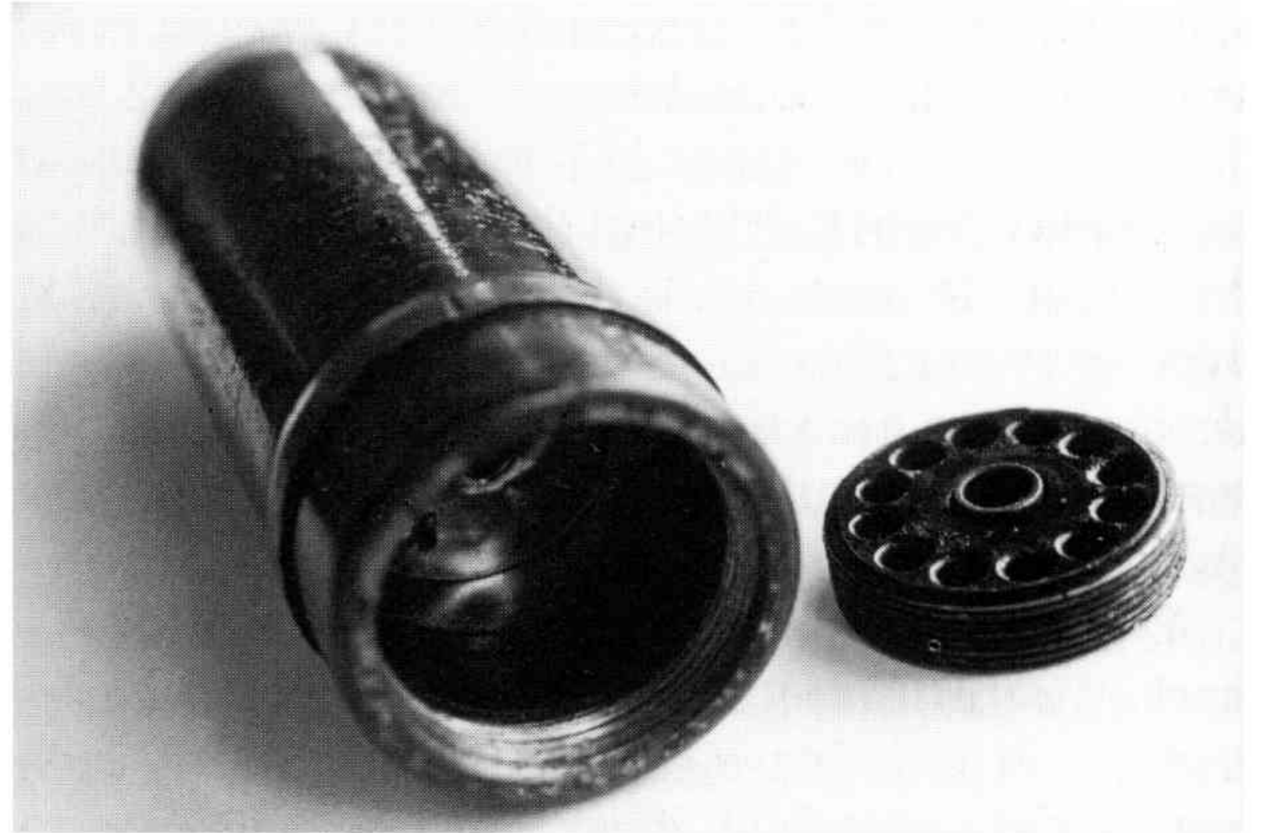
Rear of 40mm Ho-301 round with baseplate removed: note small propellant chamber and gas exhaust holes in rear plate (Courtesy: MoD Pattern Room)
