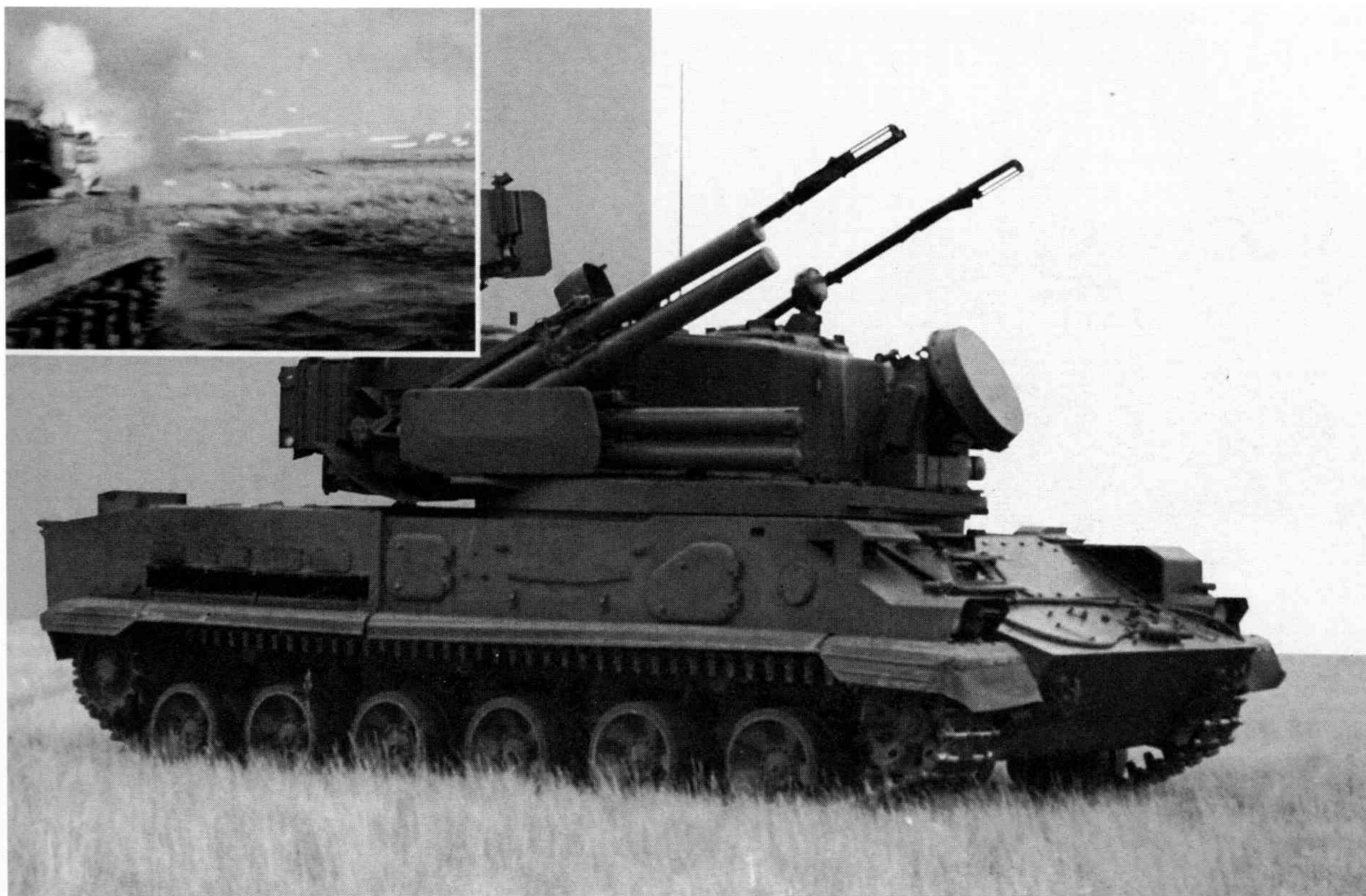
Russian Tunguska SPAAG (two twin-barrelled 30mm 2A38M, plus AA missiles) (Courtesy: Scorpion/KBP)
