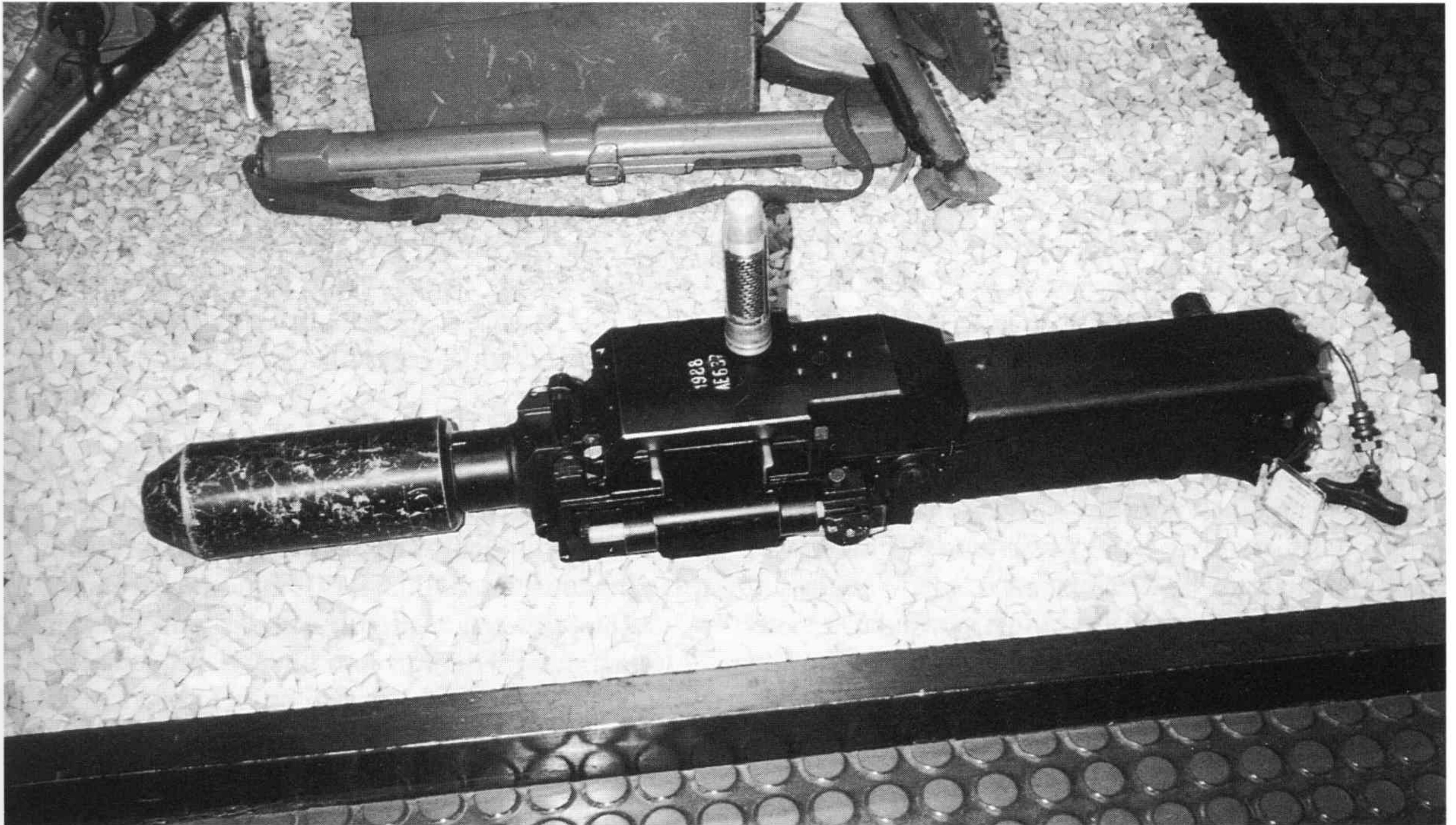
Russian 30mm AG-17A helicopter automatic grenade launcher, with round of ammunition standing on it (Courtesy: MoD Pattern Room)
