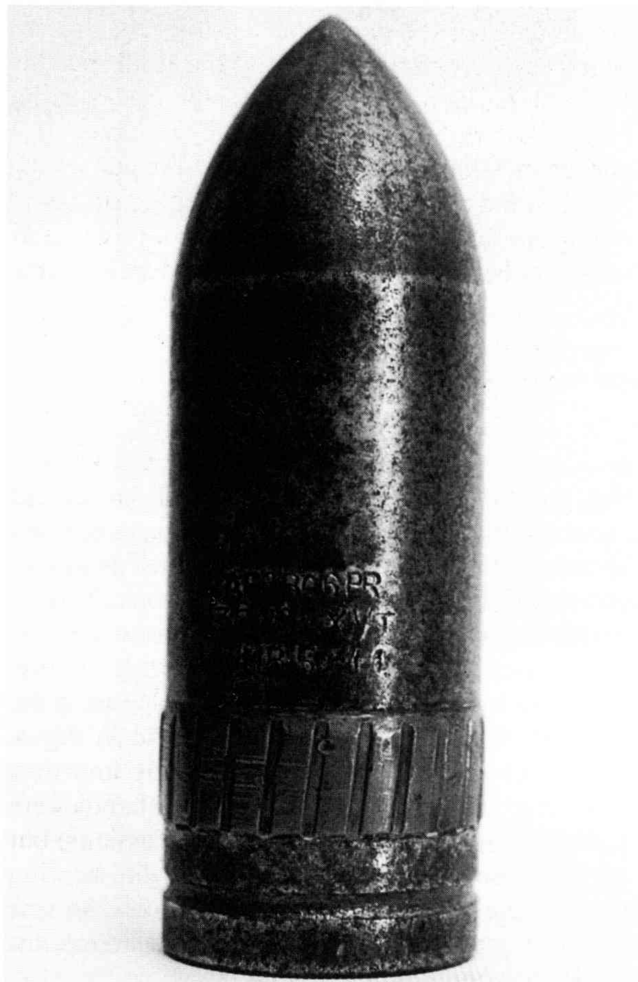
Fired 6pdr AP projectile showing driving band engraved by the rifling
