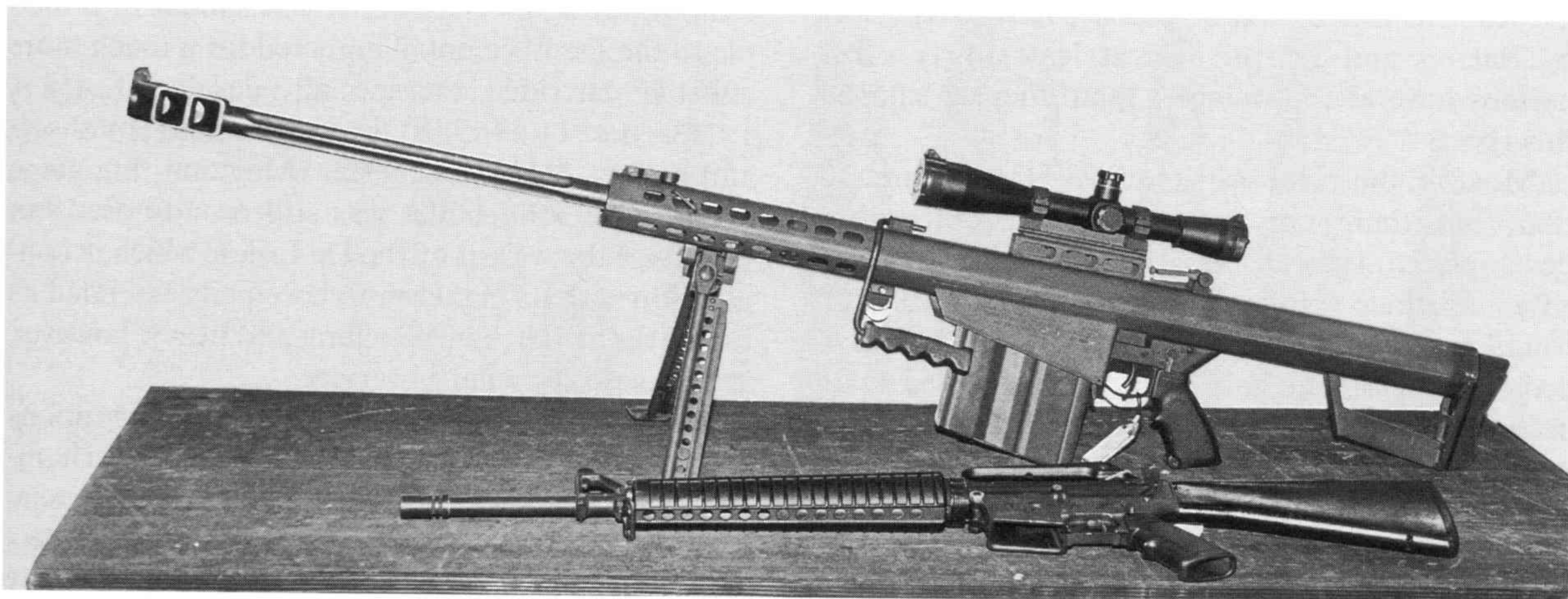
Barrett M82A1; a modern .50" calibre rifle, with M16 for scale (Courtesy: MoD Pattern Room)
