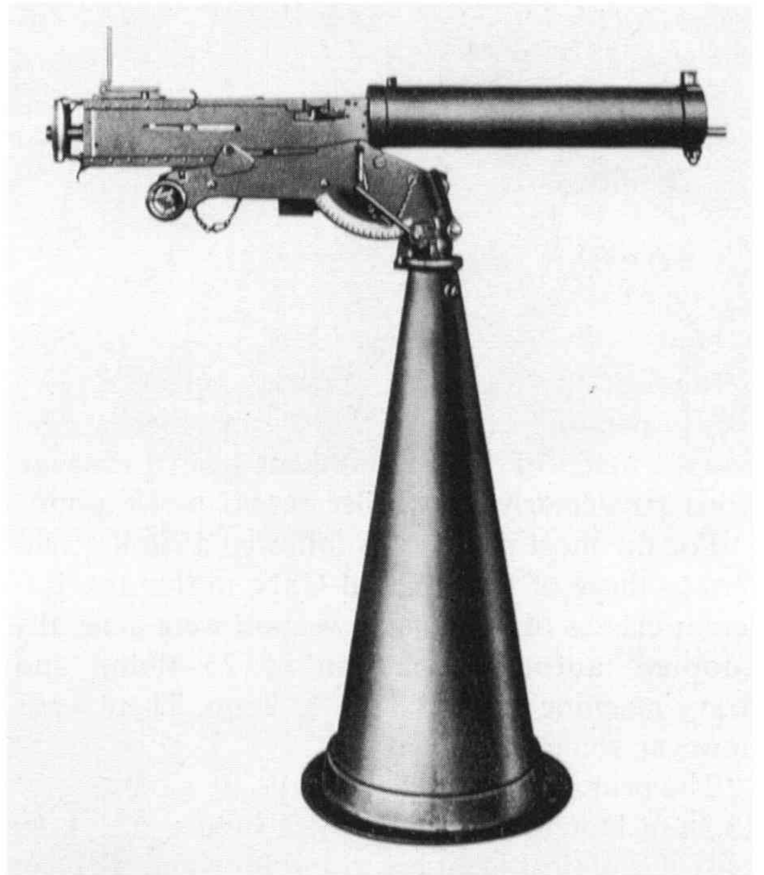
.5" Browning on pedestal mounting (Courtesy: V. Forgett)
