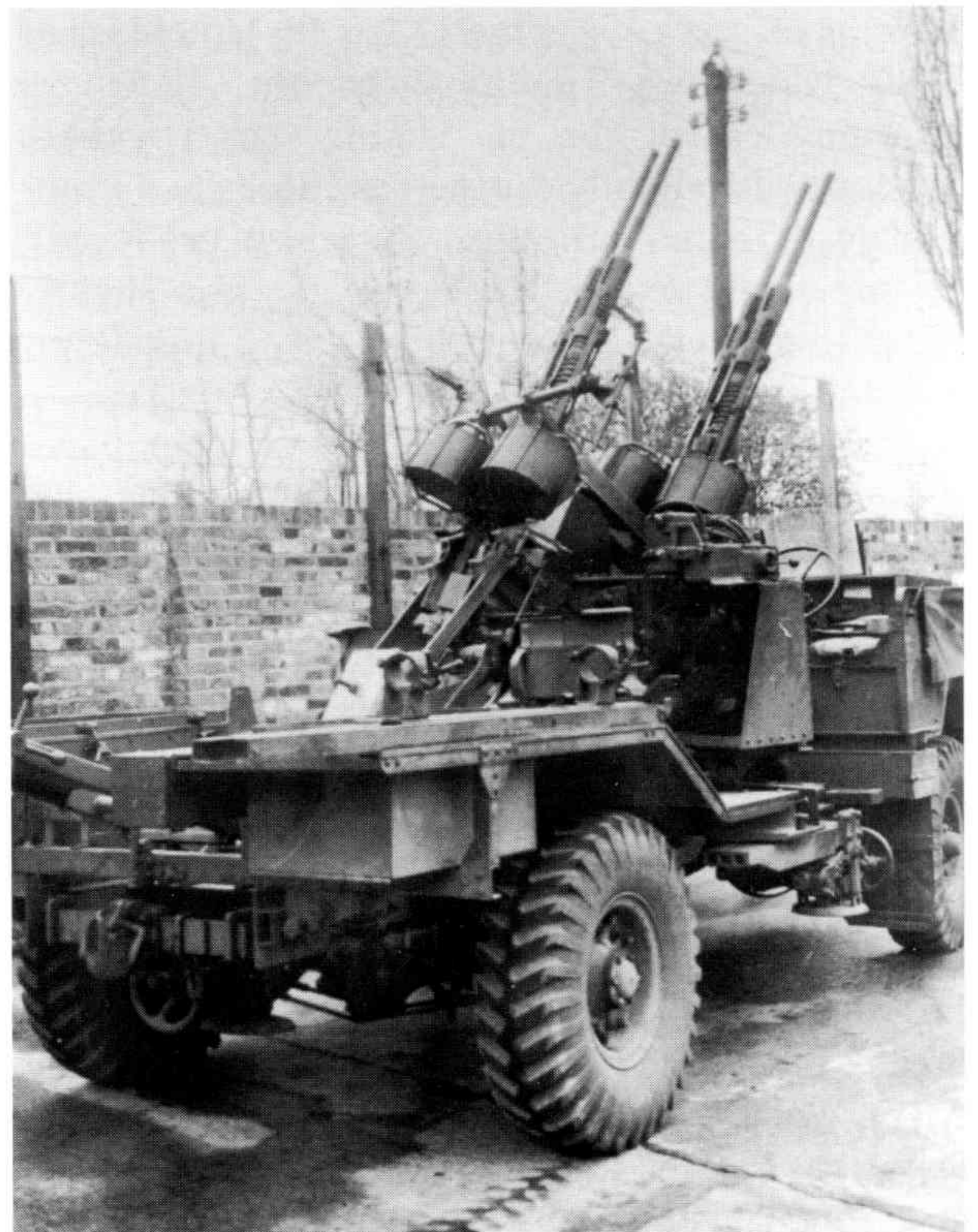
Quad 20mm Oerlikon S on British 4 × 4 mounting (Courtesy: MoD Pattern Room)
