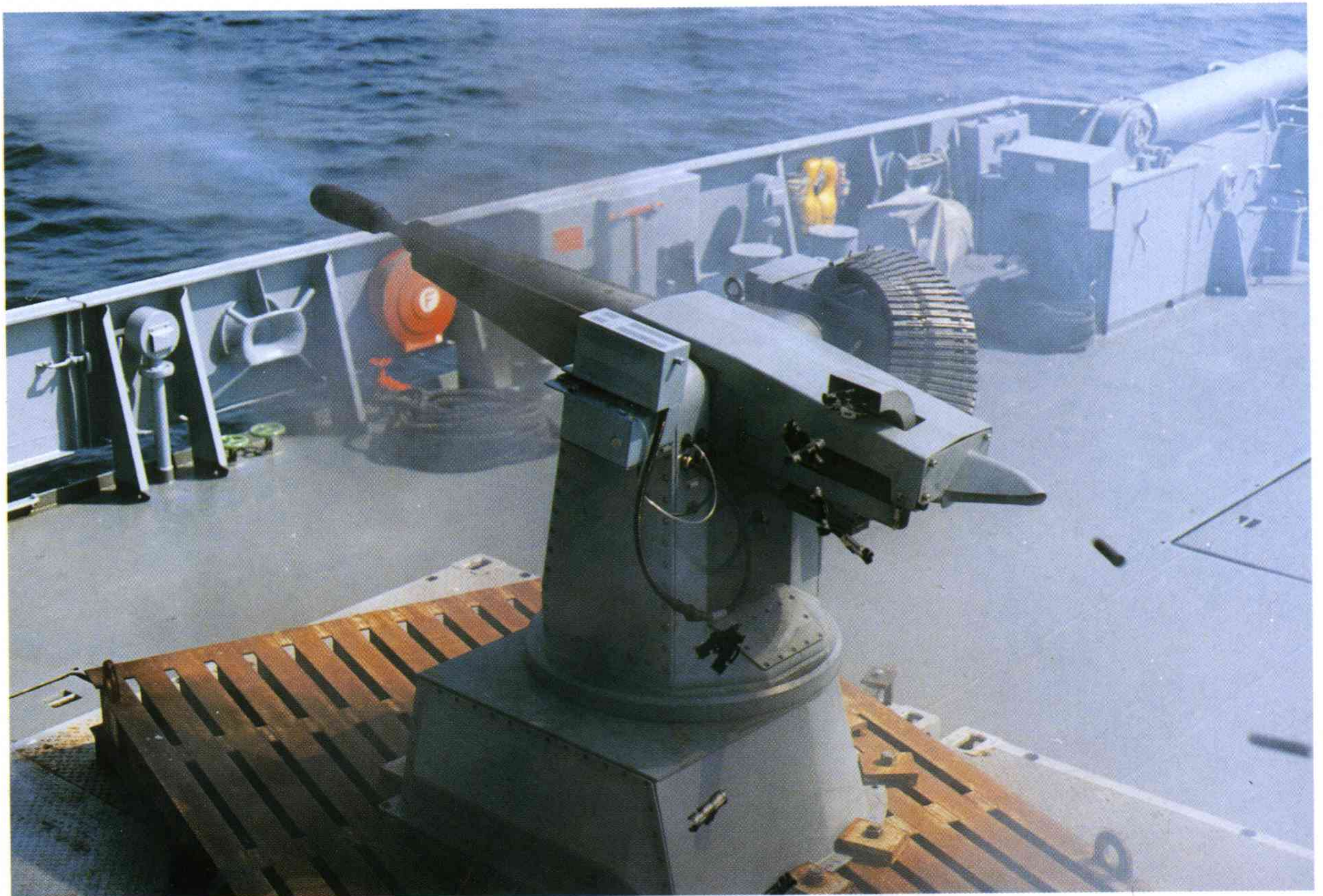
Mauser naval 27/30mm gun system during firing trials at sea (Courtesy: Mauser)
