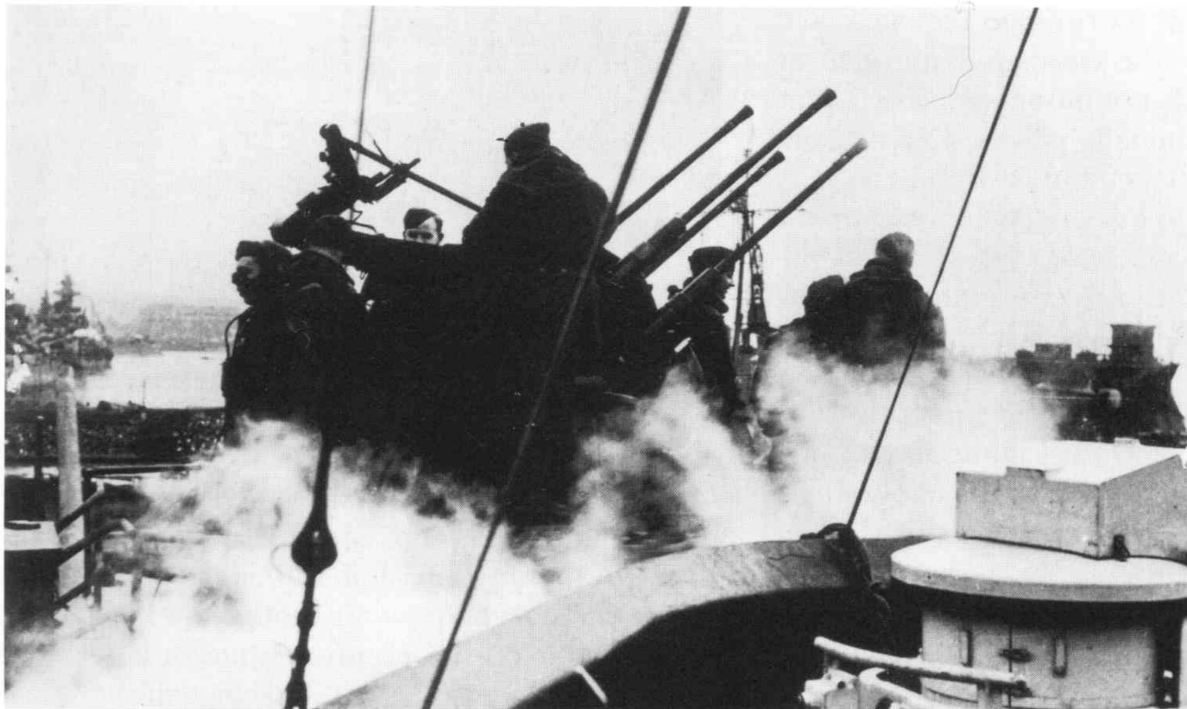
20mm Flakvierling installed on Prinz Eugen in preparation for the Channel Dash, February 1942
