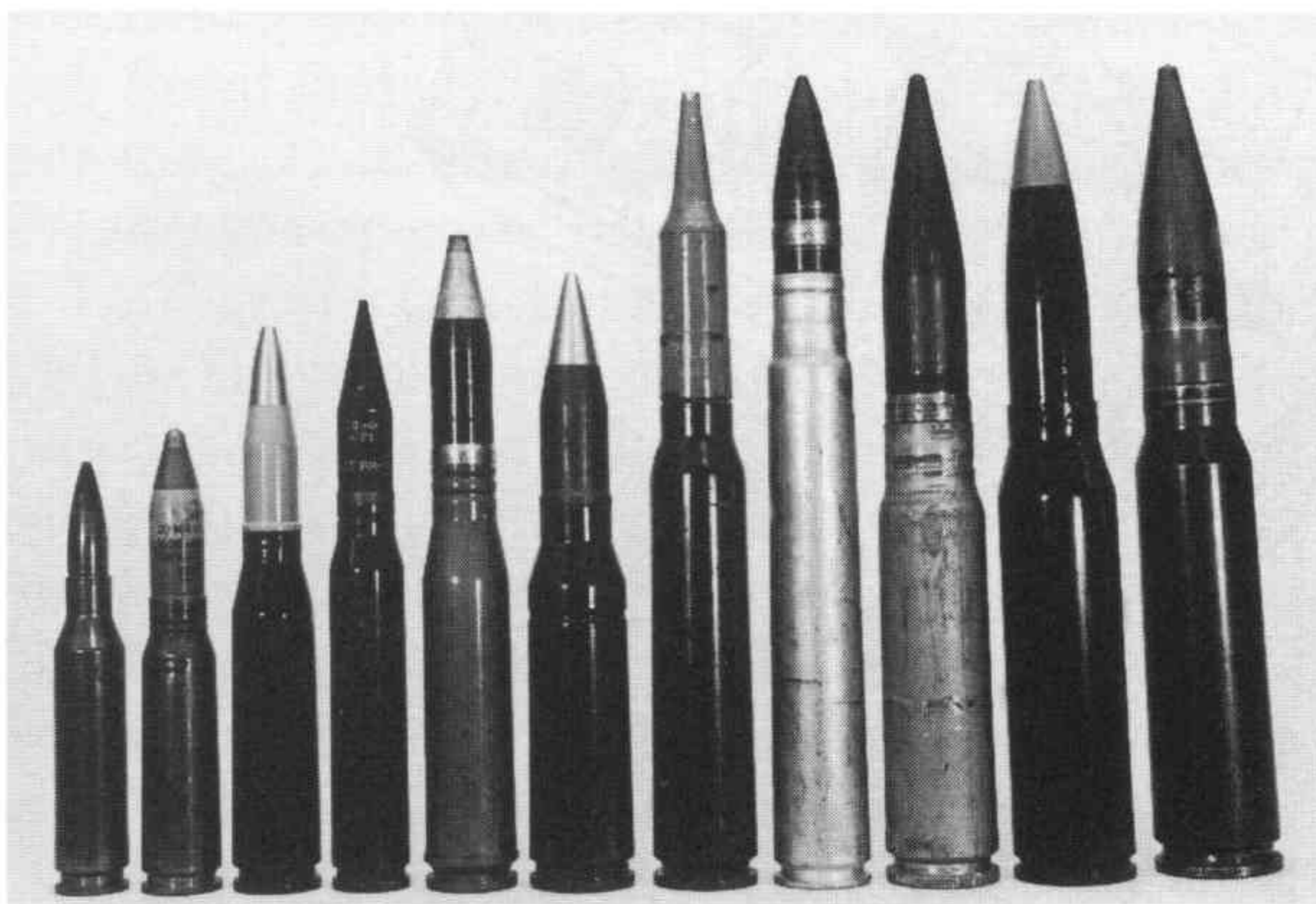
Postwar AA gun cartridges 1 (from left to right): 14.5mm KPV (14.5 × 114), 20mm M61 Vulcan (20 × 102), Oerlikon KAA (20 × 128), HS 820/Oerlikon KAD (20 × 139), 23mm ZU (23 × 152B), Oerlikon KBA/NATO (25 × 137), Oerlikon KBB (25 × 184), Soviet 2-M3/8 (25 × 218), Soviet AO-18 (30 × 165), HS 831/Oerlikon KCB (30 × 170), GAU-8/A/Mauser MK30F (30 × 173)
