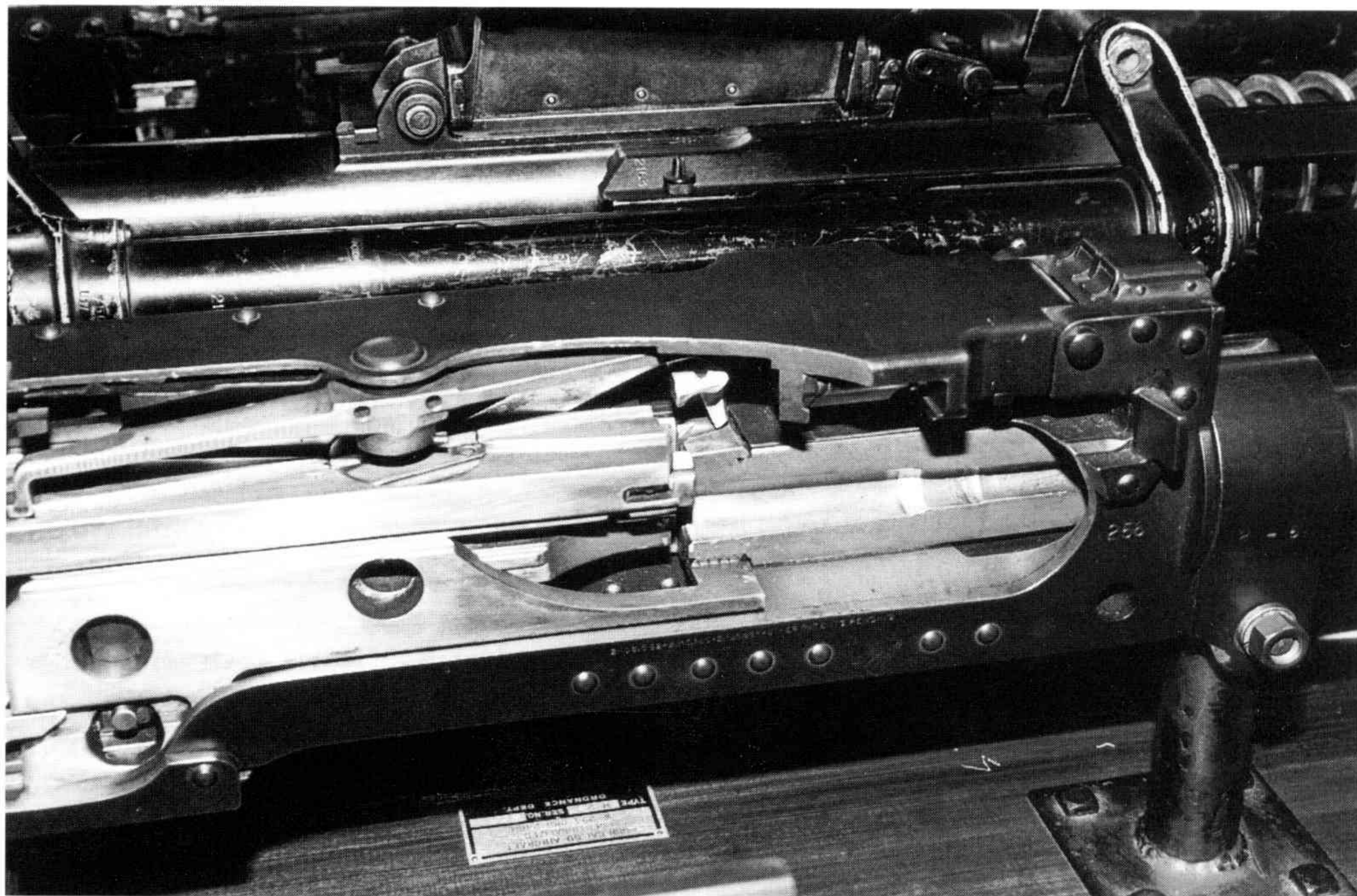
Sectioned Browning .50" M2 showing chamber (Courtesy: MoD Pattern Room)
