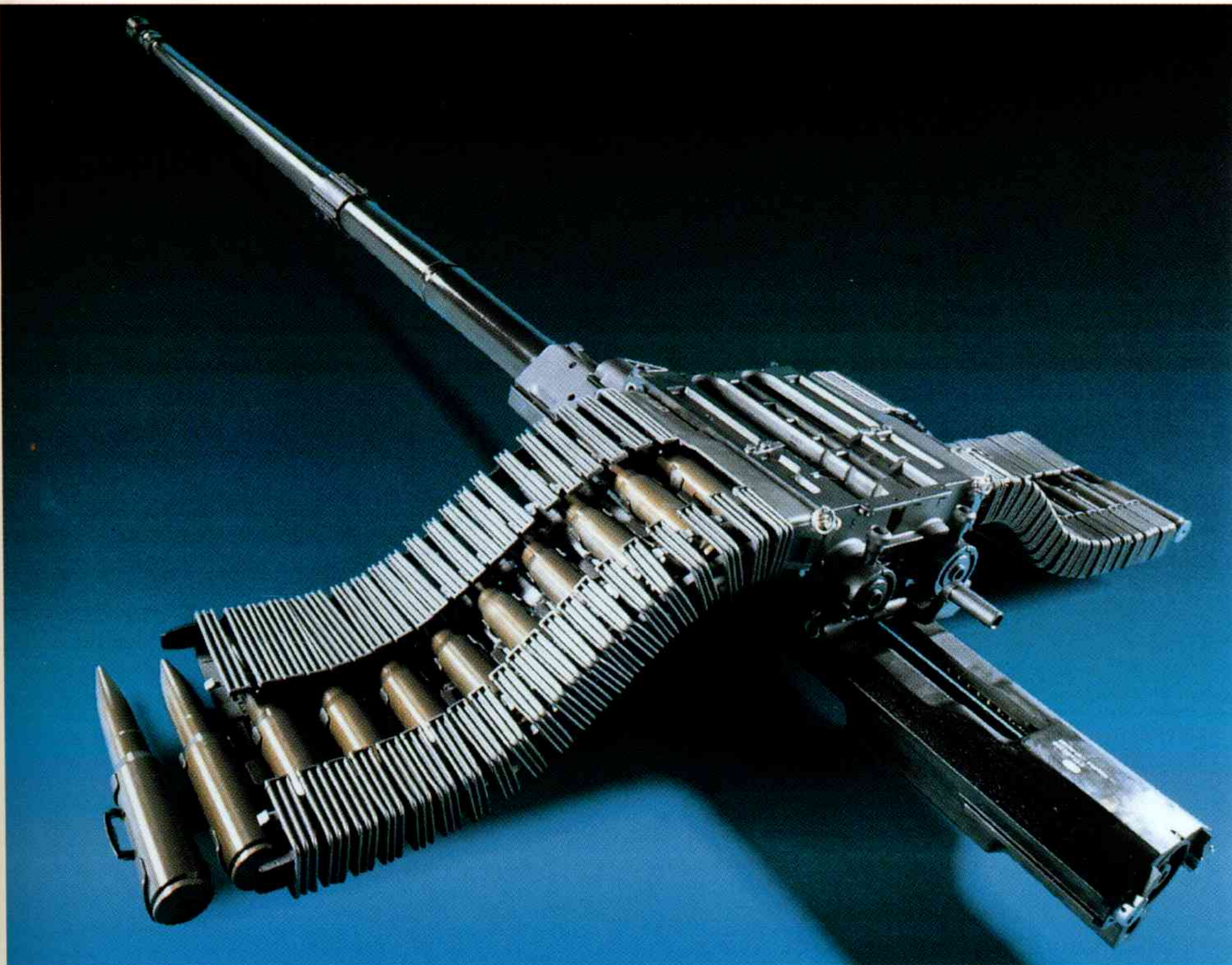
Dual belt feed with belt guides, for the Mauser MK30F (Courtesy: Mauser)
