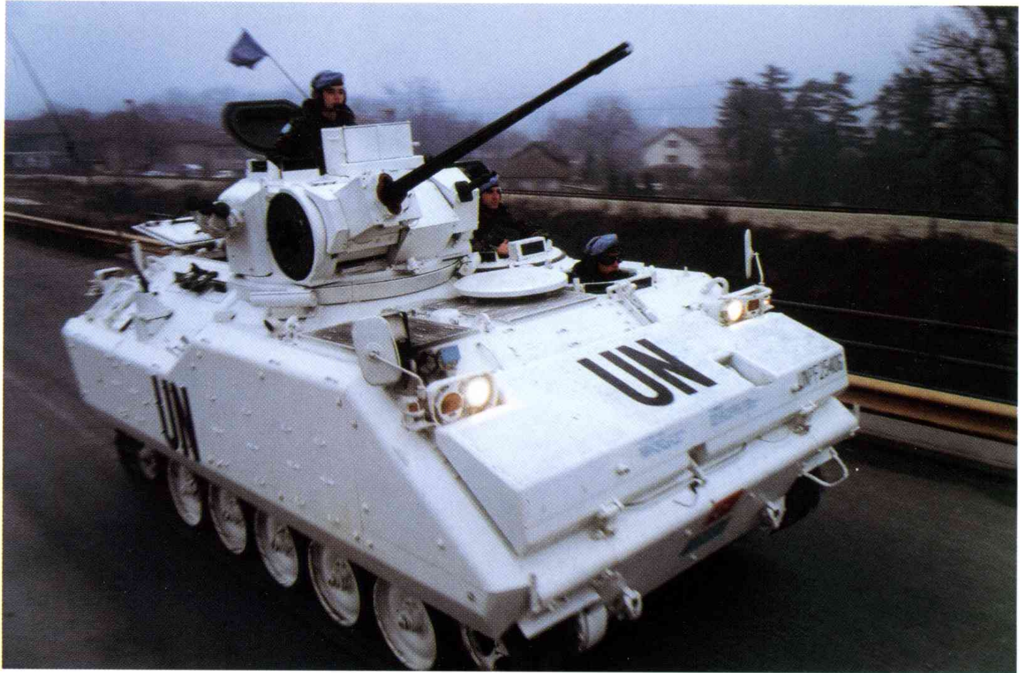
Dutch FMC AIFV with 25mm Oerlikon- Contraves KBA (Courtesy: Oerlikon- Contraves)
