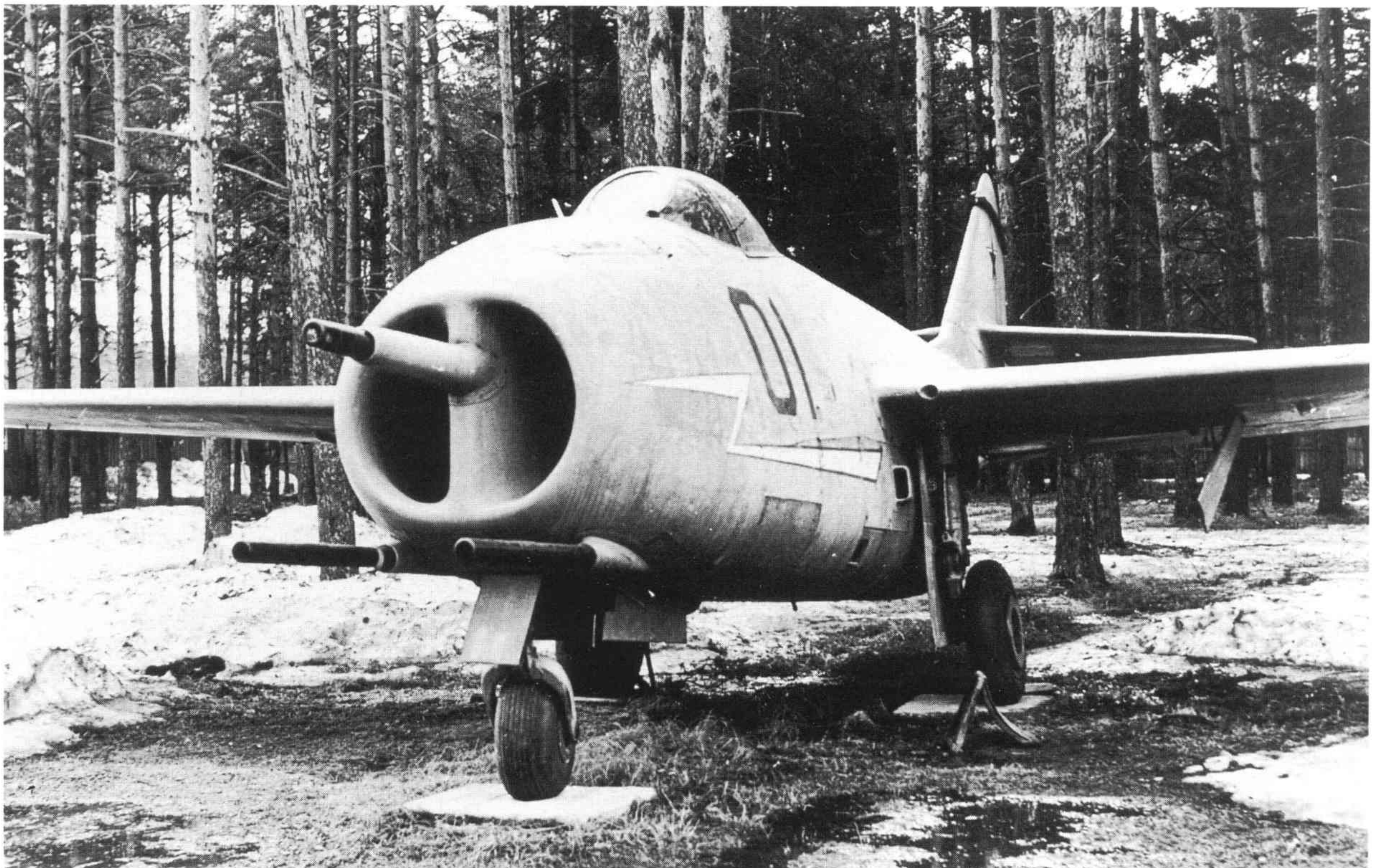
Fierce face; the MiG-9 with one N-37 and two NS-23 (Courtesy: Russian Aviation Research Trust)
