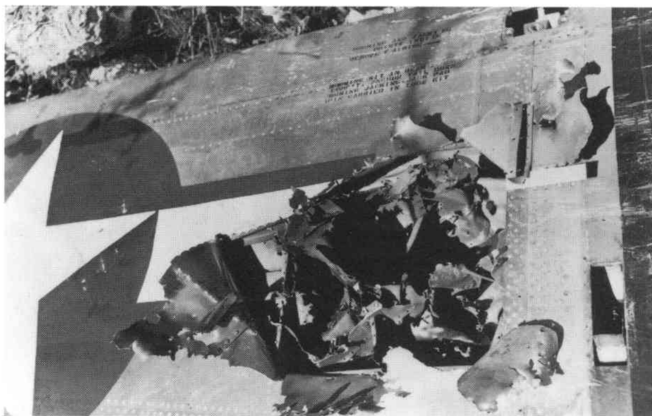
Effect of 25mm Type 96 fire; damage to P-47 wing (Courtesy: US Naval Historical Centre)
