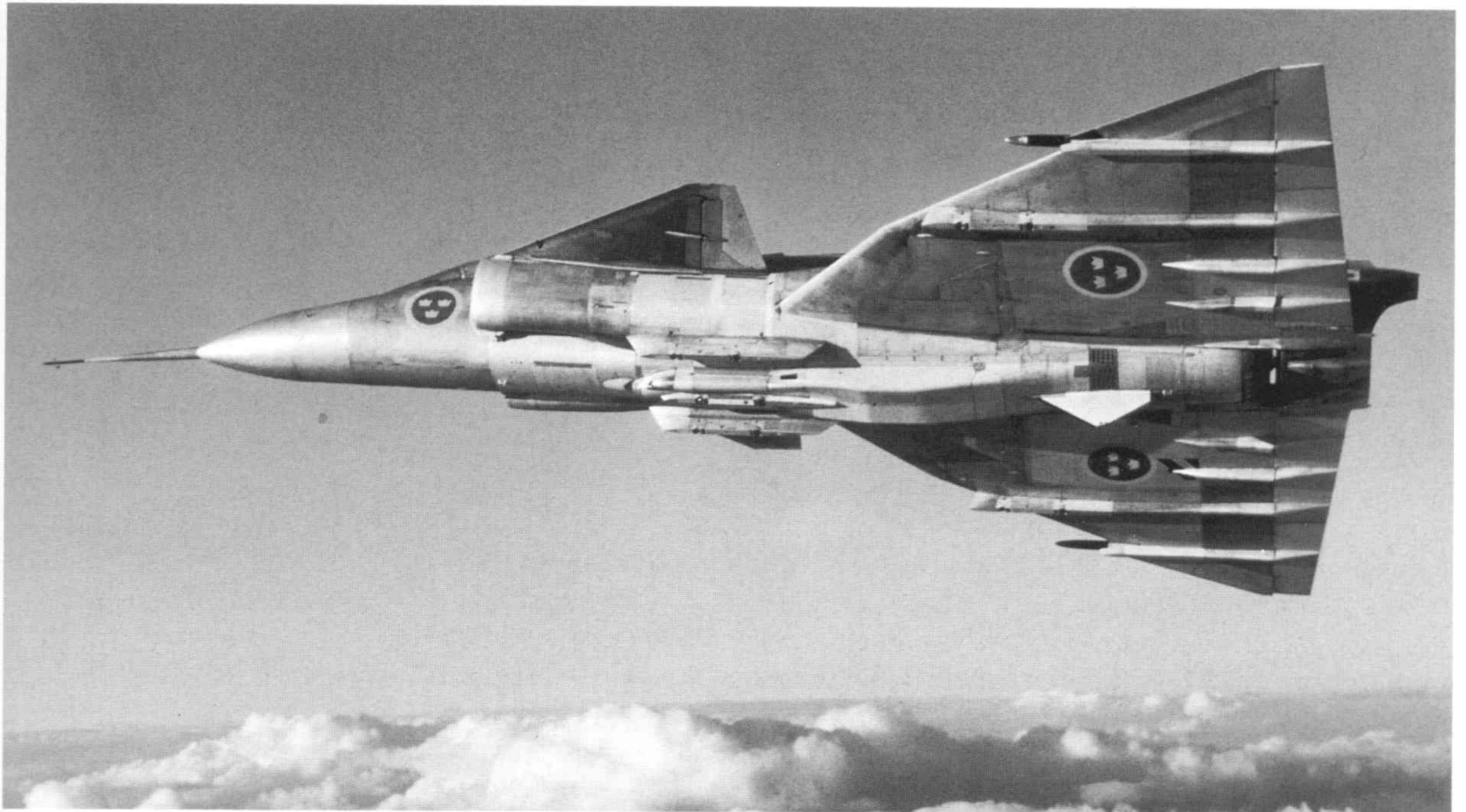
SAAB Viggen; the only aircraft with an integral 30mm Oerlikon KCA, fitted in the fairing underneath the fuselage (Courtesy: Oerlikon-Contraves)
