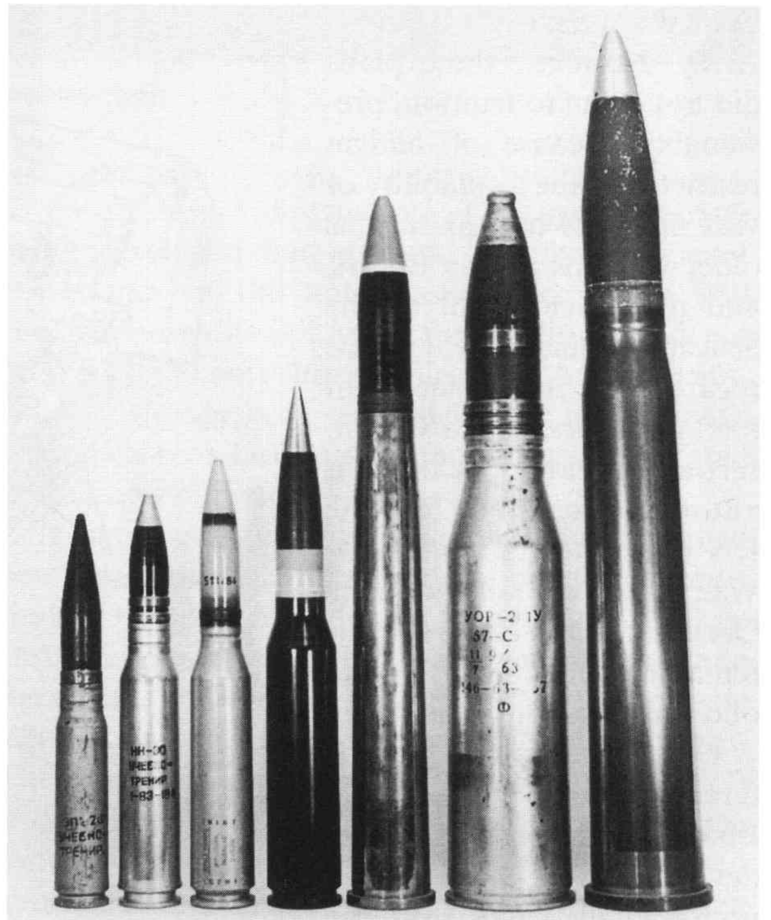
Postwar AA gun cartridges 2 (from left to right): Soviet AO-18 (30 × 165), Soviet NN-30 (30 × 210B), Czech M53 (30 × 210), Oerlikon KD/35/1000 series (35 × 228), Bofors 40mm L70 (40 × 364R), Soviet S60/ZIF 31/72 (57 × 347SR), Bofors 57mm L70 (57 × 438R)
