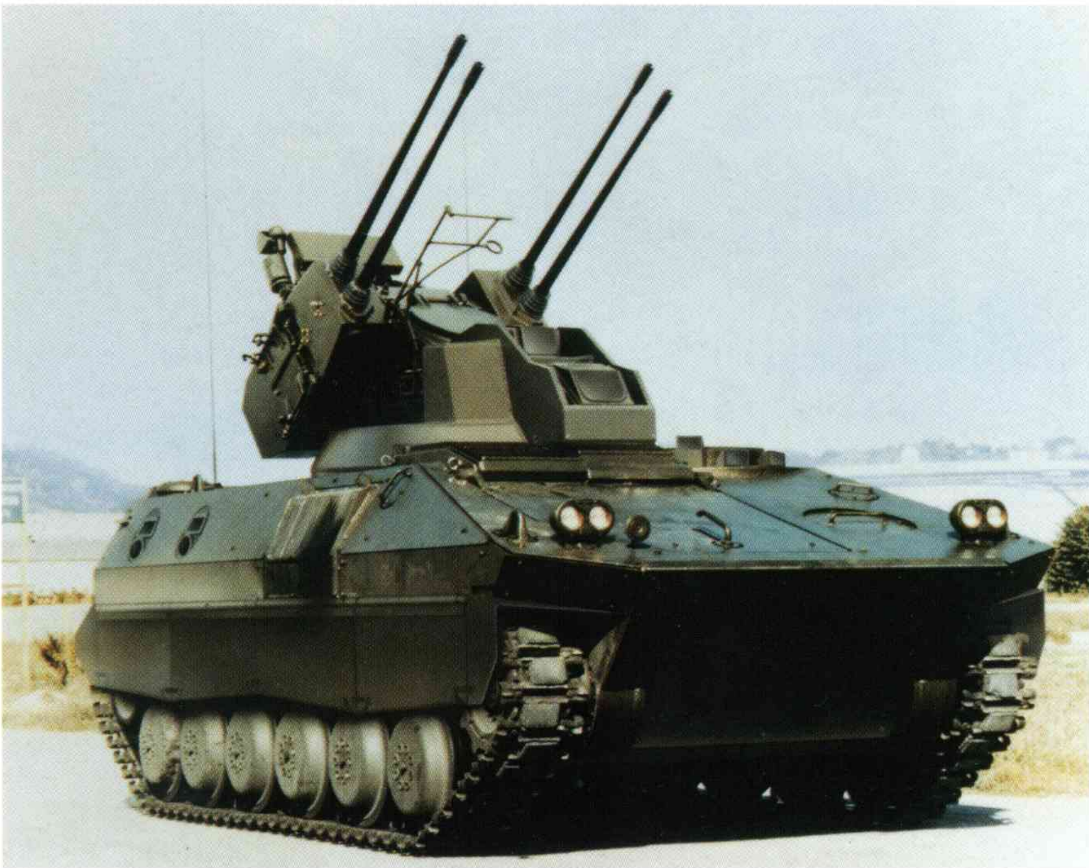
SIDAM 25 SPAAG (four 25mm Oerlikon KBA) (Courtesy: Oerlikon-Contraves)
