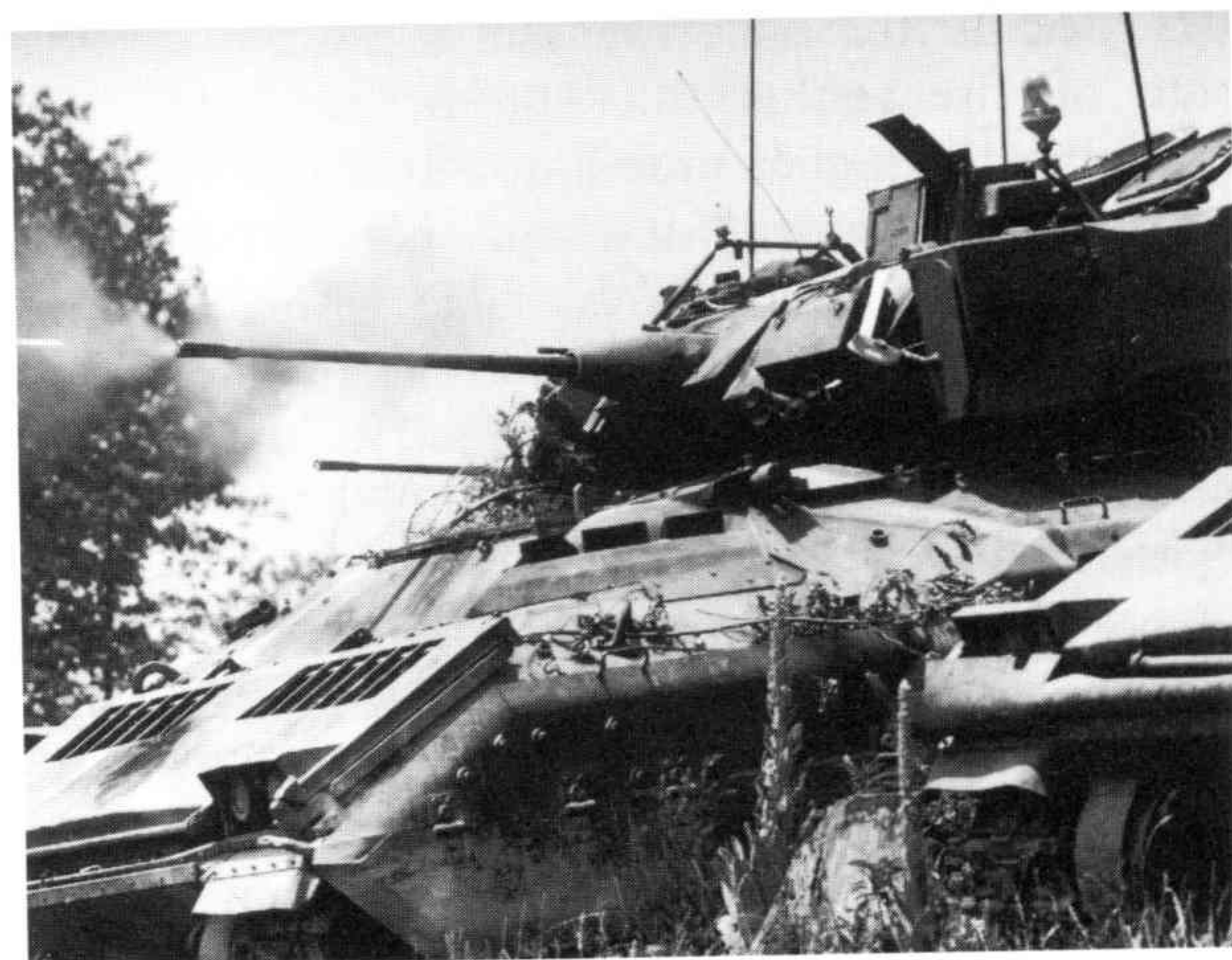
M2 Bradley MICV with 25mm Bushmaster cannon (Courtesy MDHClan Hogg)
