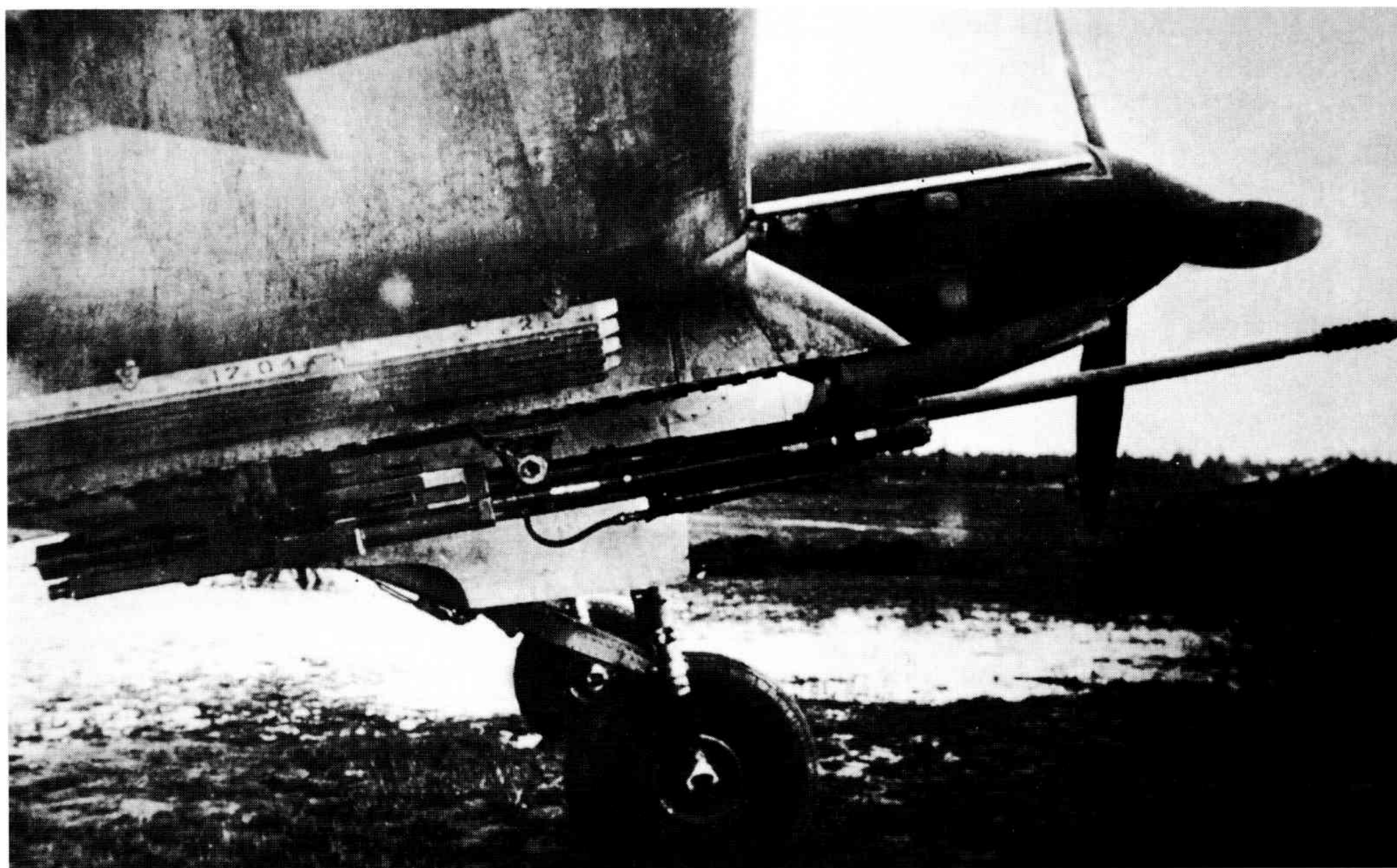
NS gun under Ilyushin Il-2 wing, with fairing removed. This appears to be the NS-45 version, as indicated by the muzzle brake. There was only one experimental installation of this gun in the Il-2 (Courtesy: Russian Aviation Research Trust)
