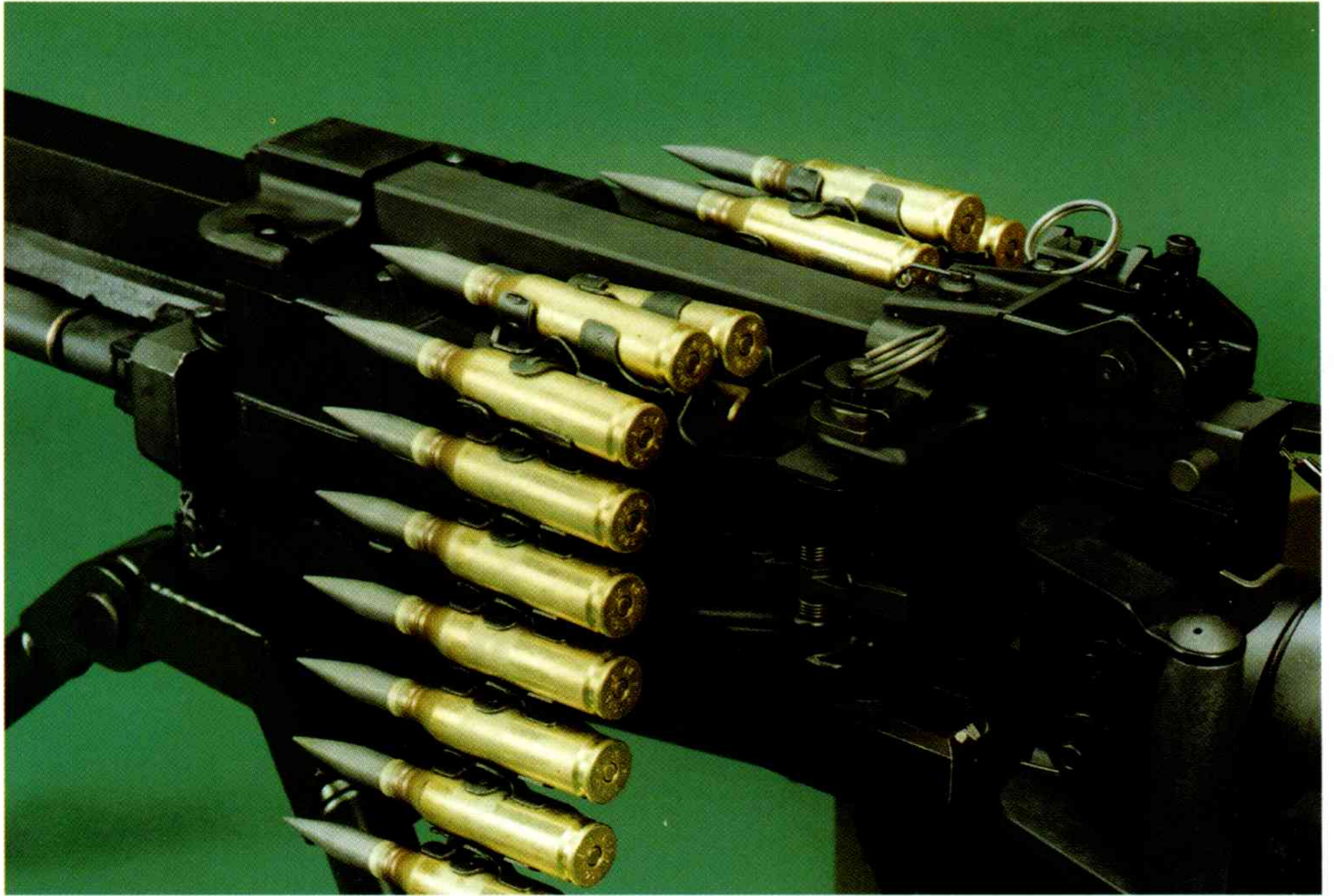
Dual belt feed, for the experimental FN-BRG 15 (Courtesy: Ian Hogg)
