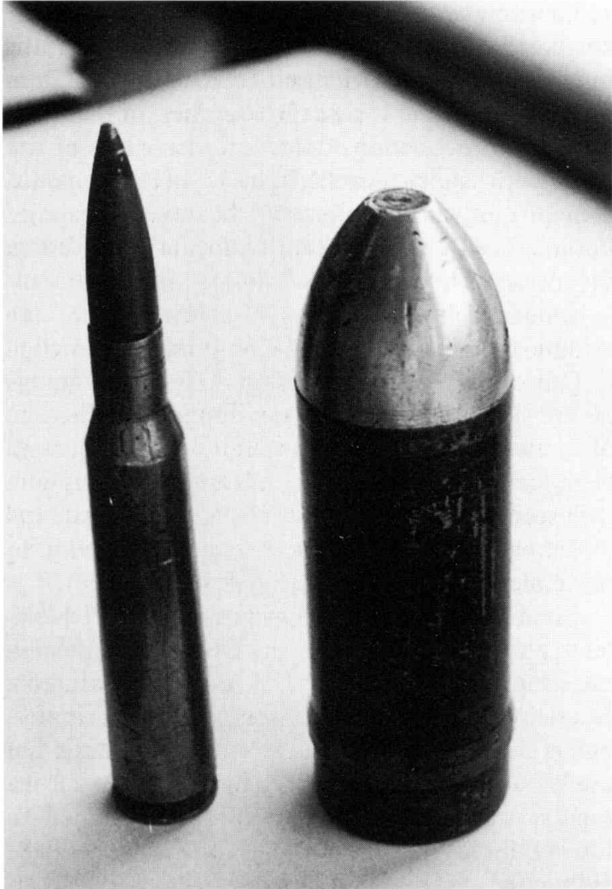
40mm caseless projectile for Ho-301 (next to 12.7 × 108 for scale) (Courtesy: MoD Pattern Room)
